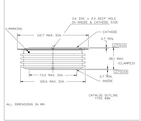
Powerex General Purpose Rectifier Diodes are designed with high locking voltage capability and low forward voltage drop to minimize conduction losses. These are packaged in hermetic, ceramic Pow-R-Disc packages which can be mounted using commercially available clamps and heatsinks or fully assembled to a variety of air or water cooled heat exchangers.
