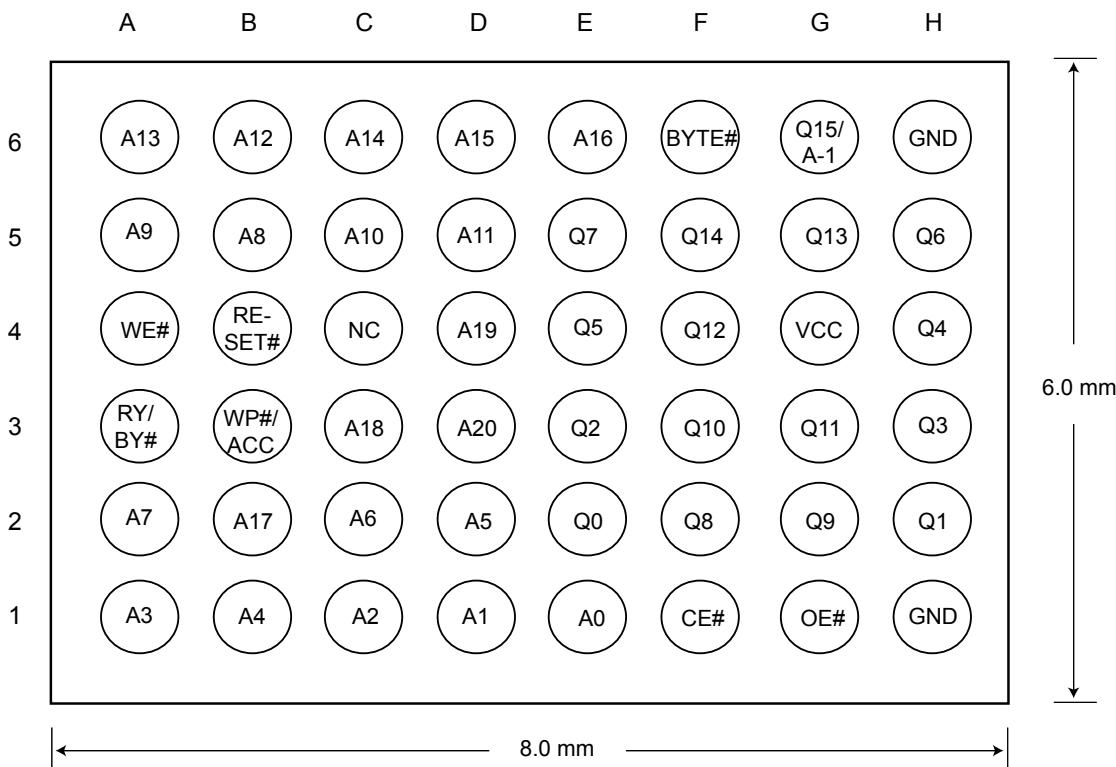
**PIN CONFIGURATION for MX29GL320E H/L**
