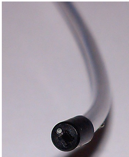
Figure 3: Distal tip of the cable with the light source and the camera
