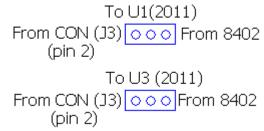
If the jumpers are placed in the left position the positive audio input will be fed from the Board Connector (J3) to the NAU82011's. In the right position the positive audio input will be taken from the NAU8402.
