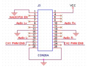
Note: CH1 PWM EN and CH2 PWM EN should be pulled to GND to Enable.
