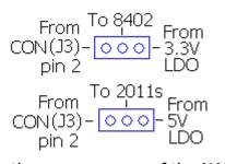
These jumpers allow the power source of the NAU82011's and the NAU8402 to be selected. In the left position the power will come from the Board Connector (J3) in the right position the power will come from the NAU83P20's onboard LDOs. Please note that while the NAU82011s can run between 2.5V and 5.5V the NAU8402 can only operate between 3V and 3.6V. *It is recommended to use the on chip LDO whenever possible.*
