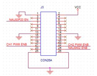
Note: CH1 PWM EN, CH2 PWM EN, and NAU8402 EN should be pulled to GND to Enable.
