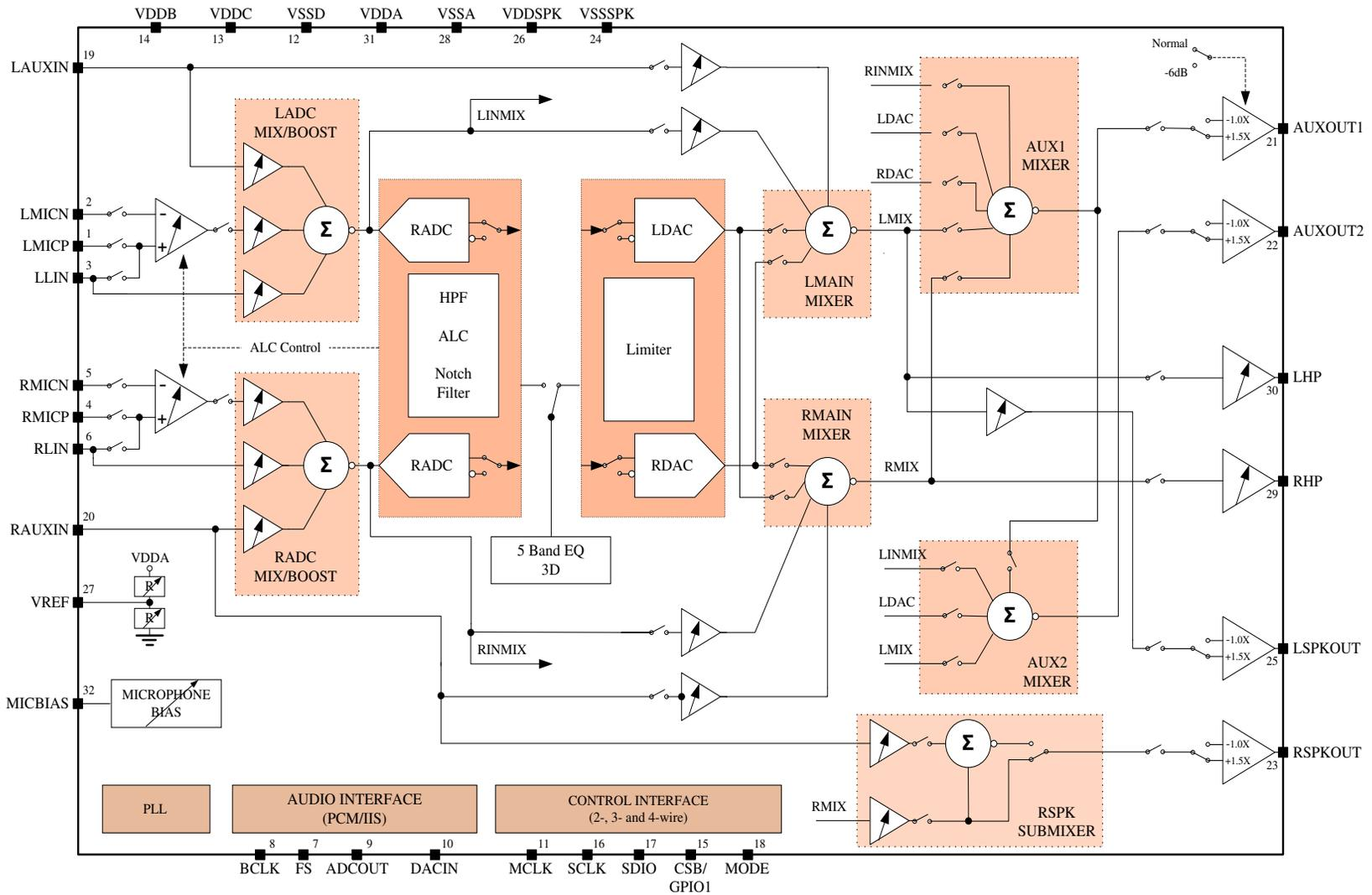
Figure 1: NAU8822ABlock Diagram
