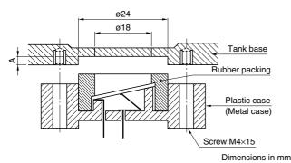
The transducer can beak off if the A dimension depth is shallow. TDK recommends a 2mm A-dimension depth and a screw tightening torque of  $0.6N \cdot m$ .
