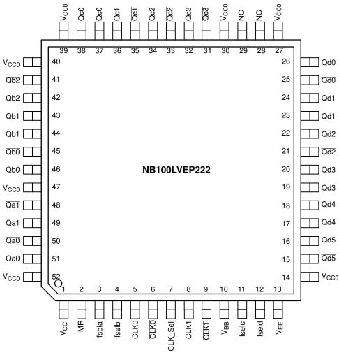
All  $V_{CC}$ ,  $V_{CC0}$ , and  $V_{EE}$  pins must be externally connected to appropriate Power Supply to guarantee proper operation.  $V_{CC}$  pin internally connected to  $V_{CC0}$  pins. The thermally conductive exposed pad on package bottom (see package case drawing) must be attached to a heat–sinking conduit. This exposed pad is electrically connected to  $V_{EE}$  internally.
