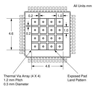
Figure 8. Recommended Solder Mask Openings
