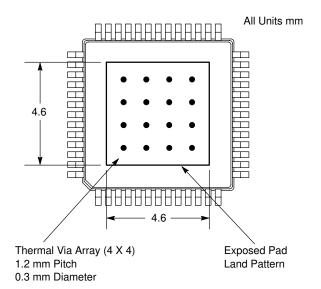
Figure 7. Recommended Thermal Land Pattern
