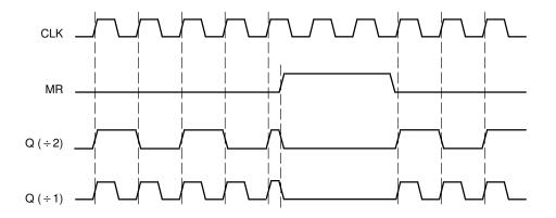
Figure 4. Master Reset (MR) Timing Diagram
