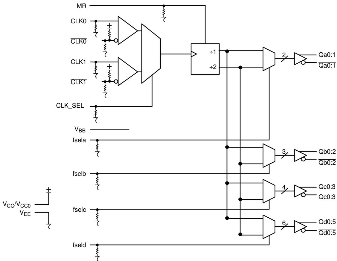
Figure 3. Logic Diagram
