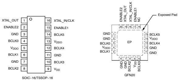
Figure 2. Pinout Configuration (Top View)
