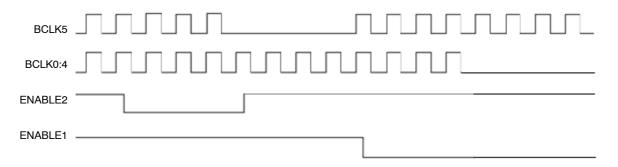
Figure 3. ENABLEx Control Timing Diagram
