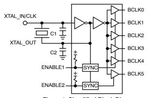
Figure 1. Simplified Block Diagram
