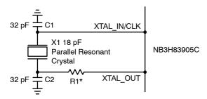
Figure 8. NB3H83905C Crystal Oscillator Interface
