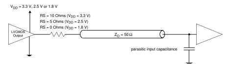
Figure 4. Application Load with Series Line Termination
