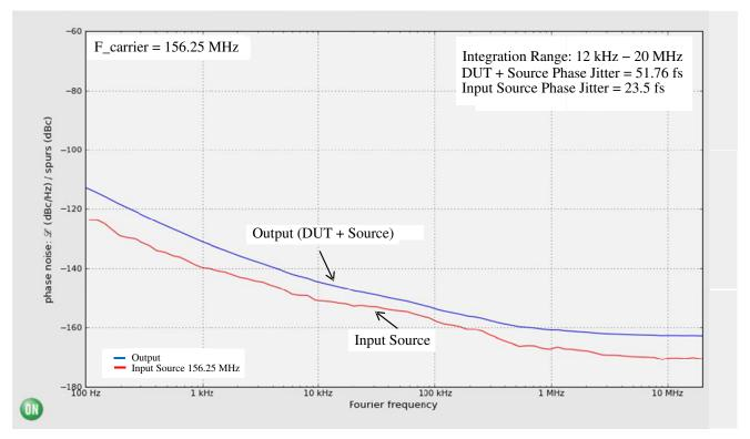
Figure 10. Typical NB3V110xC Phase Noise Plot at f<sub>Carrier</sub> = 156.25 MHz, V<sub>CC</sub> = 3.3 V V, 25°C
