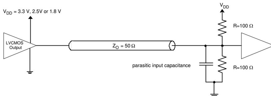
Figure 3. Application Load with 50 Ω Line Termination
