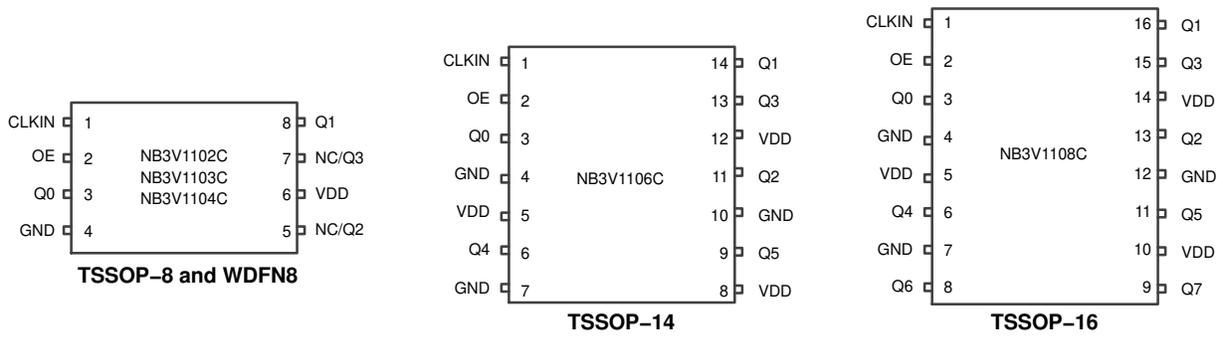
Figure 1. Pin Configuration
