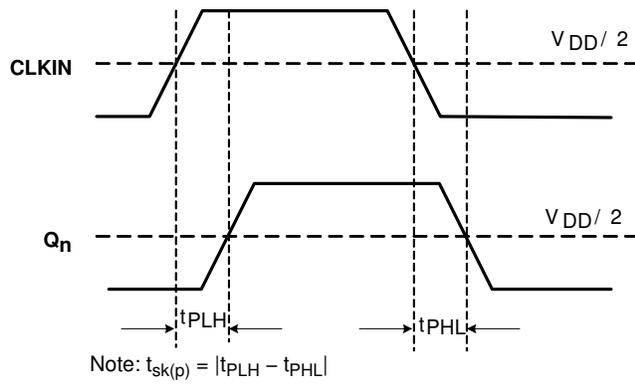
**Figure 7. Pulse Skew  $t_{sk(p)}$  and Propagation Delay  $t_{PLH}/t_{PHL}$**
