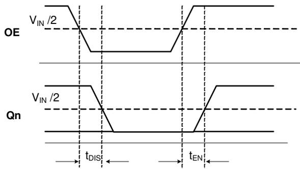
Figure 5.  $t_{DIS}$  and  $t_{EN}$  for Disable Low
