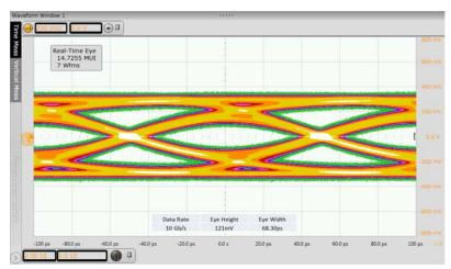
Figure 8. 10 Gbps Signal After 9 inches of FR4 at Output with Mid DE Setting to NB7NPQ702M
