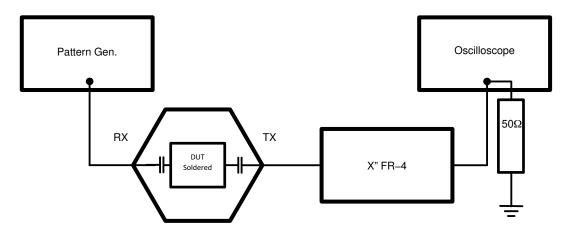
Figure 6. De-Emphasis Measurement Setup
