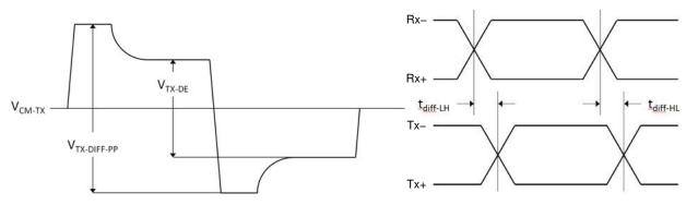
Figure 9. Transmitter Differential Voltage dB Decrease = 20 log \* (VTX-DE / VTX-DIFF-PP)
