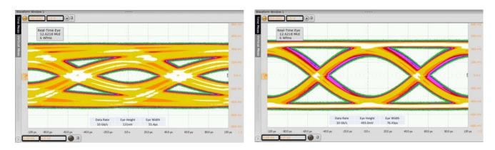
Figure 5. 10 Gbps Signal with 12 inches of FR4 Before Input to NB7NPQ702M and After with EQ Floating (Mid)
