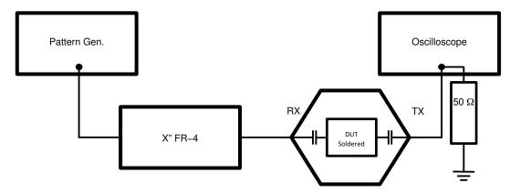
Figure 3. Equalization Measurement Setup
