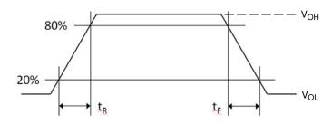
Figure 11. Output Rise and Fall Times
