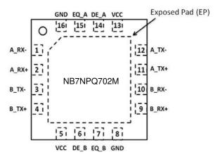
Figure 2. UQFN16 Package Pinout (Top View)
