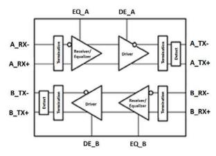
Figure 1. Logic Diagram of NB7NPQ702M
