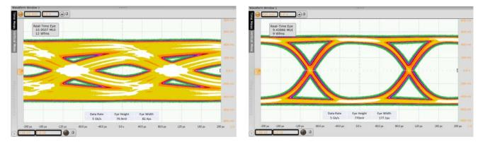
Figure 4. 5 Gbps Signal with 24 inches of FR4 Before Input to NB7NPQ702M and After Using High EQ Setting
