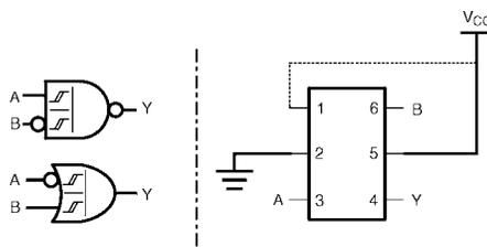
FIGURE 3. 2-Input NAND with Inverted B Input
