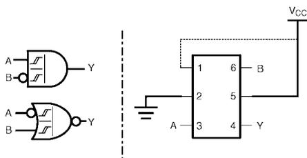
FIGURE 8. 2-Input AND with Inverted B Input
