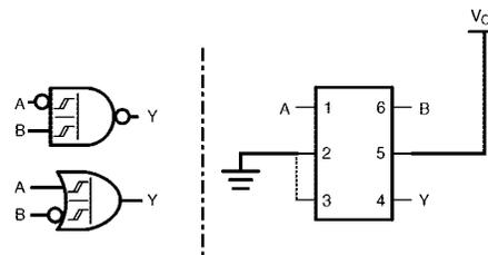
FIGURE 2. 2-Input NAND with Inverted A Input
