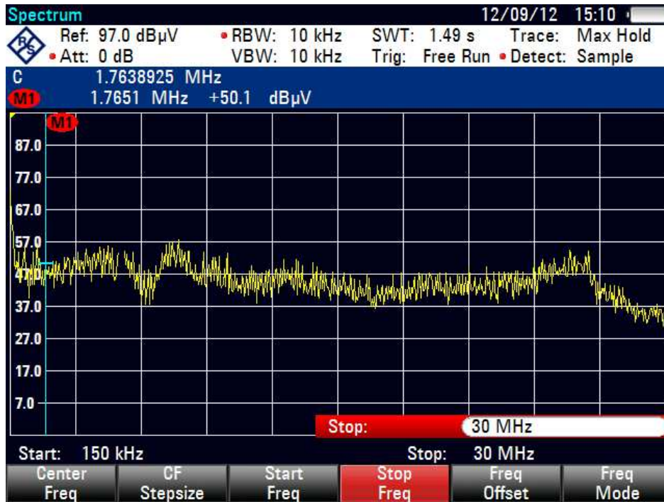
Figure 30. Conducted EMI Pre-compliance 150 kHz–30 MHz
