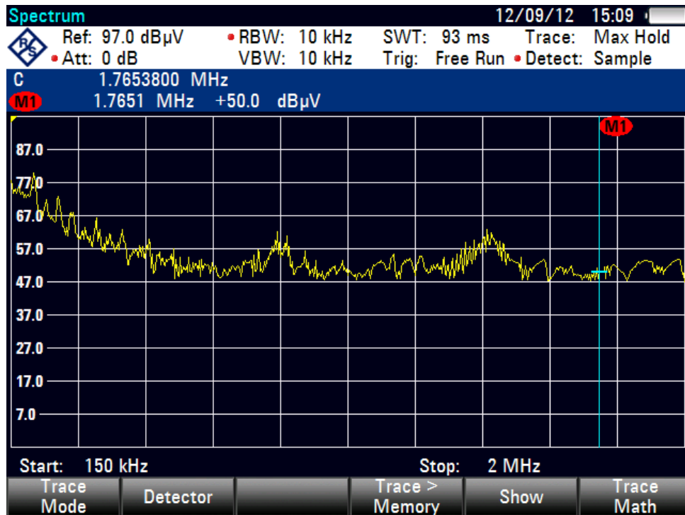
Figure 29. Conducted EMI Pre-compliance 150 kHz-2 MHz
