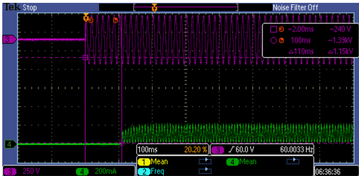
Figure 16. Start Up with AC Applied 230 V Maximum Load
