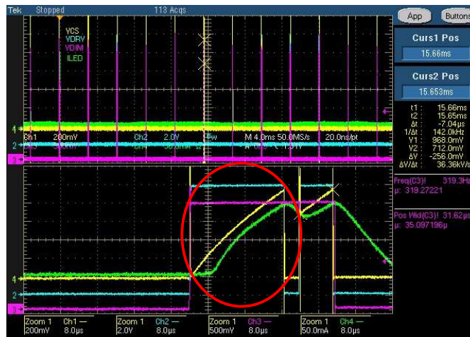
Figure 31. Minimum Dimming Duty Cycle
