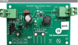
enables the use of a pulsewidth modulated logic signal to dim the LED directly. The soft-start pin creates a startup sequence that slowly ramps up the peak current and enables the adjustment of the peak current set point for analog dimming control. The device features robust protection features to detect switch overcurrent faults and to detect maximum on time events.
