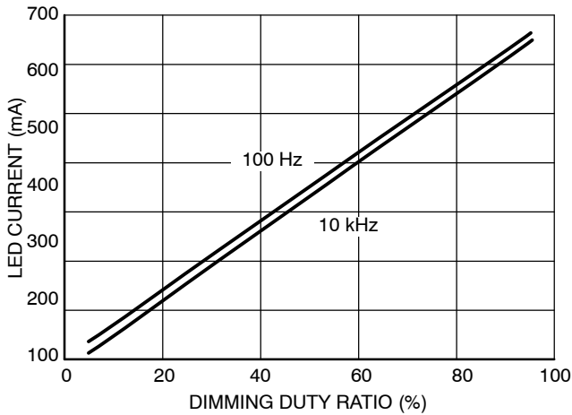
Figure 13. LED Current vs. Dimming Duty Ratio
