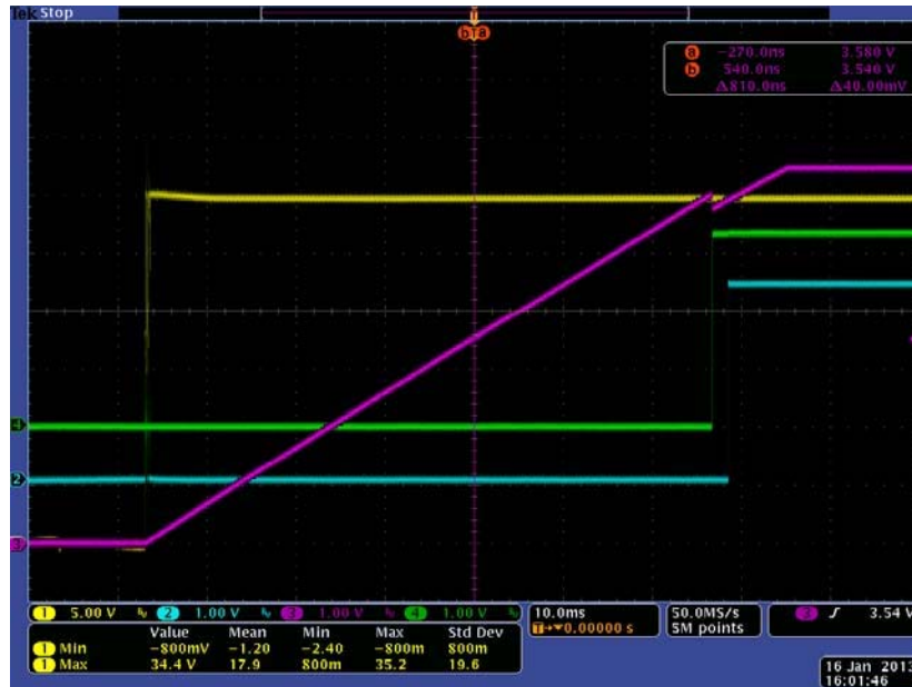
Figure 6. NCN5150 Startup Sequence
