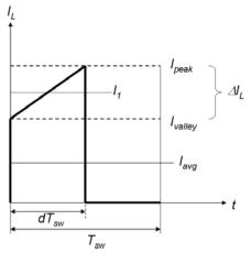
Figure 43. Primary Inductance Current Evolution in CCM
