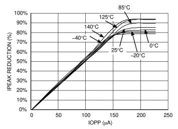
Figure 22. Ipeak Reduction = F(lopp, @ temperature)
