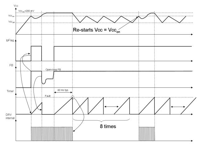
Figure 26. In case of short–circuit or overload, the NCP1028 protects itself and the power supply via a low frequency burst mode. The V<sub>CC</sub> is maintained by the current source and self–supplies the controller.
