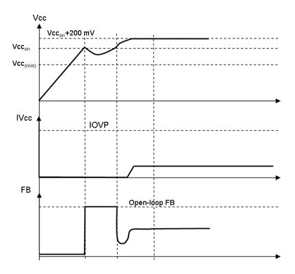
Figure 24. A typical startup sequence showing the V<sub>CC</sub> capacitor voltage evolution versus time.
