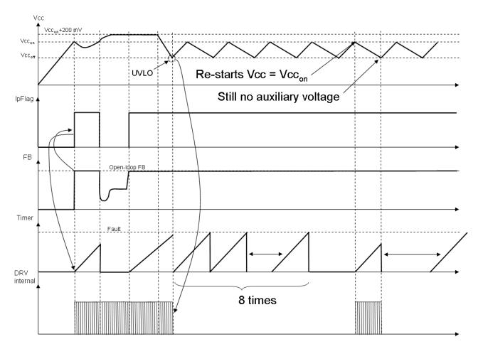
Figure 27. The auxiliary winding collapses in presence of a short-circuit. Pulses are immediately stopped as  $V_{CC}$  crosses the minimum operating voltage,  $VCC_{(min)}$ .
