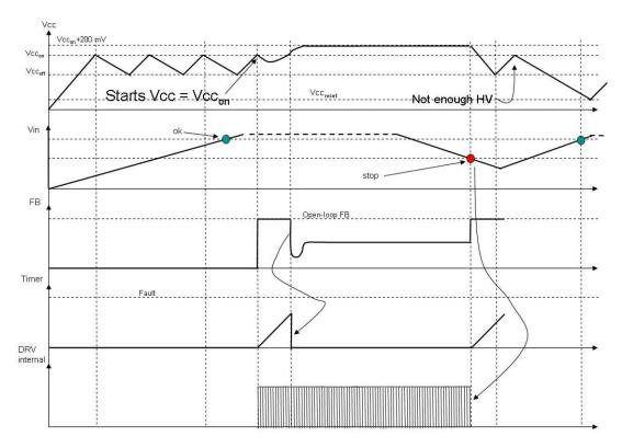
Figure 30. Signal Evolution During a Brown-Out Condition
