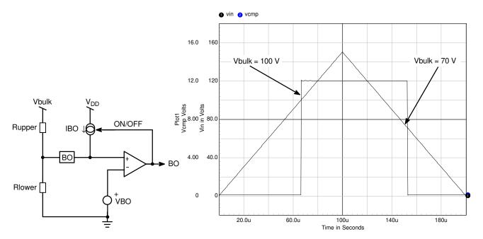
Figure 29a. The internal brown-out configuration with an offset current source.
