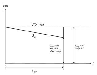
Figure 38. Maximum Peak Current Setpoint Variations versus Ramp Compensation
