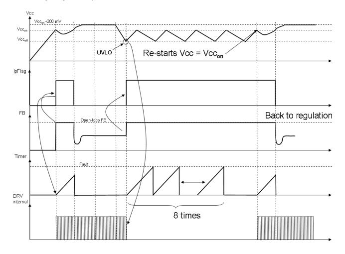
Figure 28. In this particular case, the output goes low but the timer is not started since the FB pin is still held by the optocoupler. Due to the UVLO circuit, the controller safely stops operation at  $V_{CC} = VCC_{(min)}$ .
