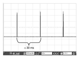
Figure 34. The burst frequency becomes so low that it is difficult to keep an adequate level on the auxiliary V<sub>CC</sub>.
