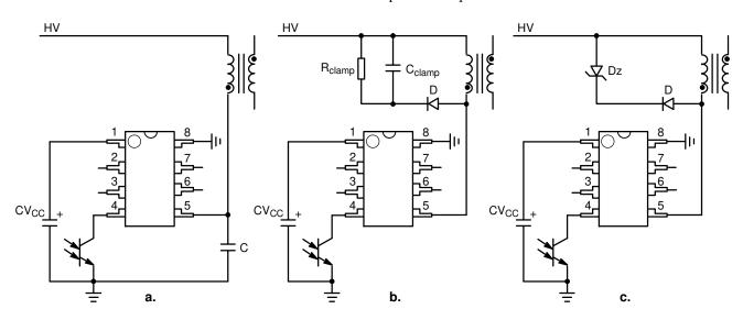
Figure 44. Different Options to Clamp the Leakage Spike
