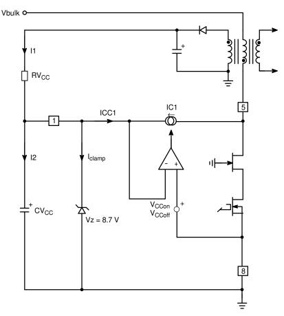
Figure 23. Internal Arrangement of the Startup Circuitry
