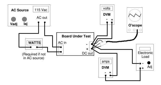
Note: Indicated output polarity on above drawing of demo board may not correspond to actual demo board. Please note output polarity as marked on demo board behind the output terminal strip.
