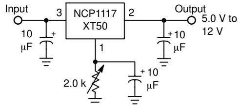
Figure 32. Adjusting Output of Fixed Voltage Regulators
