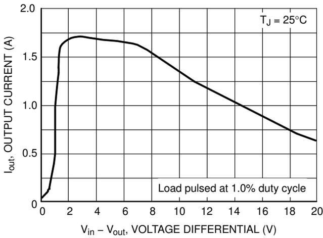
**Figure 6. Output Short Circuit Current vs. Differential Voltage**
