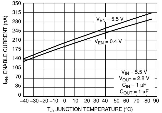
Figure 18. Current to Enable Pin vs. Temperature
