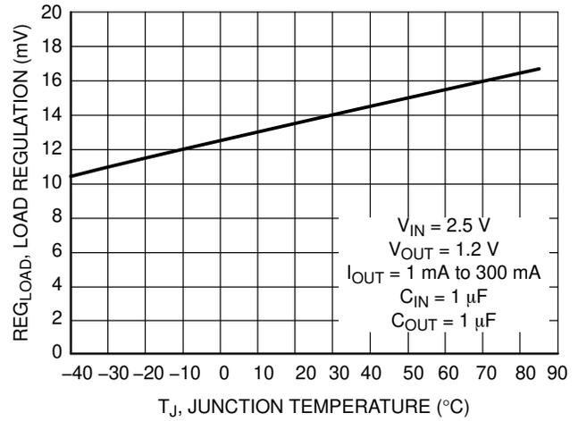
Figure 10. Load Regulation vs. Temperature
