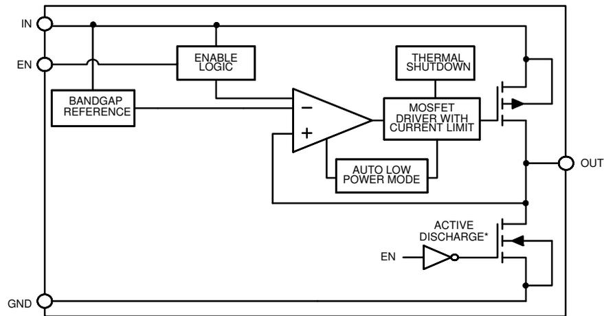
\*Active output discharge function is present only in NCP114AMXyyyTCG devices.
