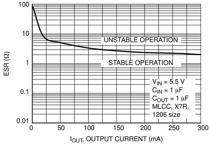
Figure 25. Output Capacitor ESR vs. Output Current
