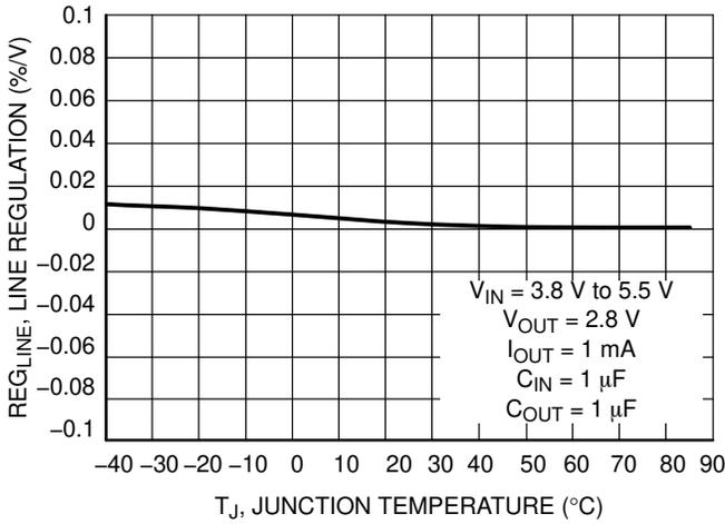
Figure 9. Line Regulation vs. Temperature
