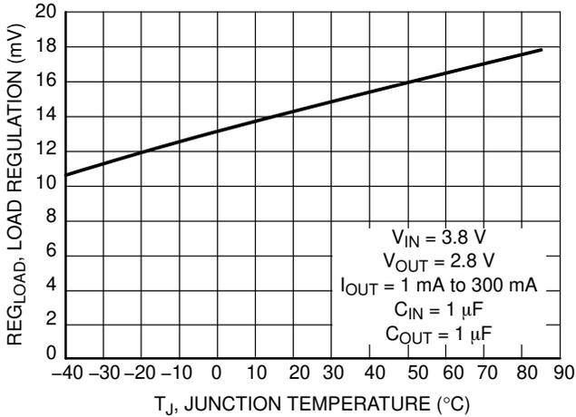
Figure 11. Load Regulation vs. Temperature
