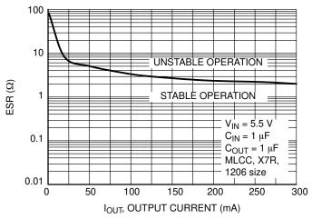
Figure 25. Output Capacitor ESR vs. Output Current
