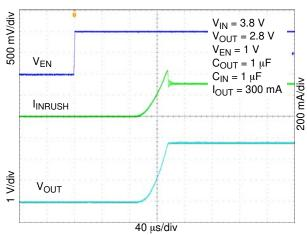
Figure 27. Enable Turn-on Response,  $C_{OUT} = 1 \mu F$ ,  $I_{OUT} = 300 \text{ mA}$
