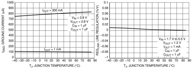
Figure 7. Ground Current vs. Temperature
