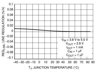
Figure 9. Line Regulation vs. Temperature  $V_{OUT} = 2.8 \text{ V}$
