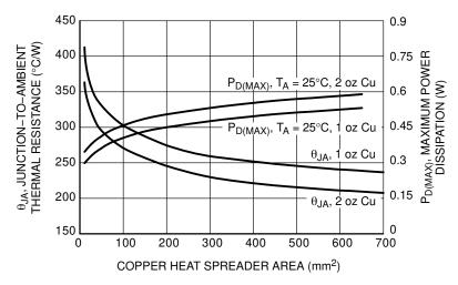
Figure 43. θ<sub>JA</sub> vs. Copper Area (TSOP-5)
