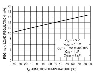
Figure 10. Load Regulation vs. Temperature  $V_{OUT} = 1.2 \text{ V}$
