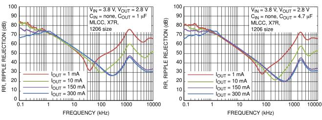
Figure 23. Power Supply Rejection Ratio,  $V_{OUT}$  = 2.8 V,  $C_{OUT}$  = 1  $\mu F$
