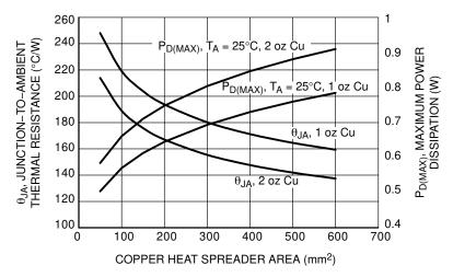
Figure 42. θ<sub>JA</sub> vs. Copper Area (uDFN4)
