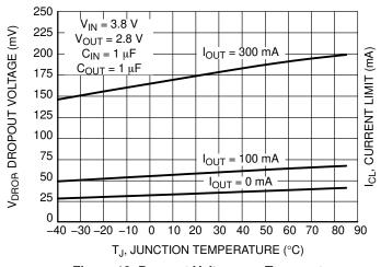
Figure 13. Dropout Voltage vs. Temperature
