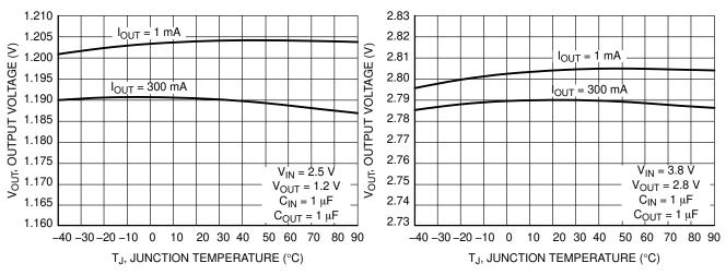
Figure 3. Output Voltage vs. Temperature  $V_{OUT} = 1.2 \text{ V}$
