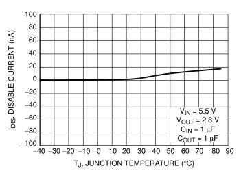
Figure 19. Disable Current vs. Temperature
