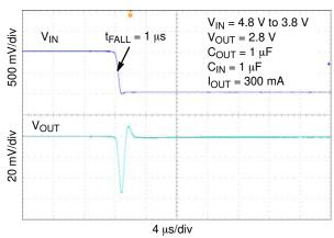
Figure 33. Line Transient Response – Falling Edge, V<sub>OUT</sub> = 2.8 V, I<sub>OUT</sub> = 300 mA
