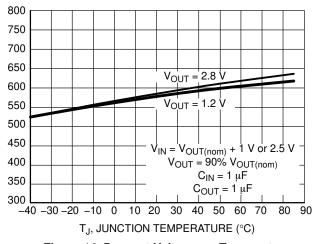
Figure 14. Dropout Voltage vs. Temperature
