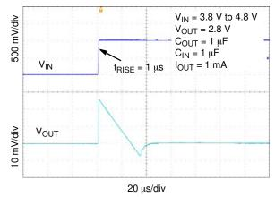
Figure 30. Line Transient Response – Rising Edge,  $V_{OUT}$  = 2.8 V,  $I_{OUT}$  = 1 mA
