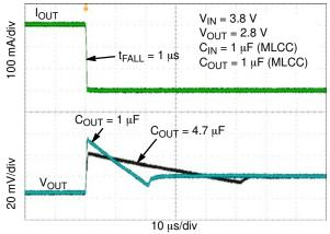
Figure 37. Load Transient Response – Falling Edge,  $V_{OUT}$  = 2.8 V,  $I_{OUT}$  = 1 mA to 300 mA,  $C_{OUT}$  = 1  $\mu$ F, 4.7  $\mu$ F
