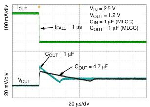
Figure 35. Load Transient Response – Falling Edge,  $V_{OUT}$  = 1.2 V,  $I_{OUT}$  = 1 mA to 300 mA,  $C_{OUT}$  = 1  $\mu$ F, 4.7  $\mu$ F
