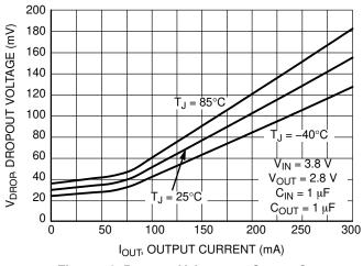
Figure 12. Dropout Voltage vs. Output Current V<sub>OUT</sub> = 2.8 V
