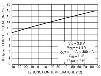
Figure 11. Load Regulation vs. Temperature V<sub>OUT</sub> = 2.8 V
