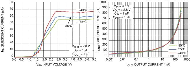
Figure 5. Quiescent Current vs. Input Voltage
