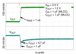
Figure 34. Load Transient Response – Rising Edge,  $V_{OUT}$  = 1.2 V,  $I_{OUT}$  = 1 mA to 300 mA,  $C_{OUT}$  = 1  $\mu$ F, 4.7  $\mu$ F
