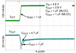
Figure 36. Load Transient Response – Rising Edge,  $V_{OUT}$  = 2.8 V,  $I_{OUT}$  = 1 mA to 300 mA,  $C_{OUT}$  = 1  $\mu$ F, 4.7  $\mu$ F
