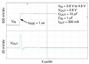
Figure 32. Line Transient Response – Rising Edge, V<sub>OUT</sub> = 2.8 V, I<sub>OUT</sub> = 300 mA
