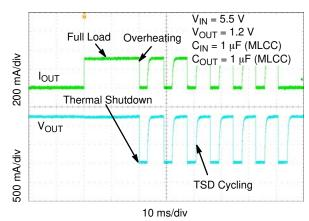
Figure 41. Short–Circuit and Thermal Shutdown
