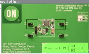
inverting and step-down applications. This device is available in space-saving thin SOT23-5 (TSOP-5) package. With its small footprint, the device is also ideal for generating a boosted voltage from a 3.3 V or 5.0 V power rail.
