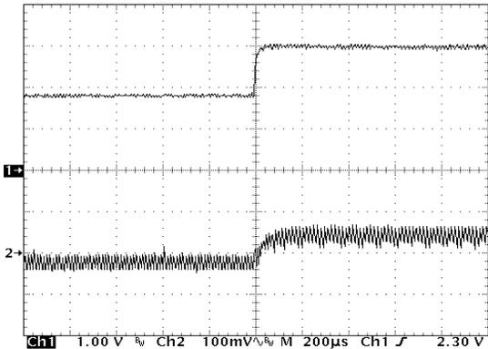
( $V_{IN} = 1.8\text{ V}$ , to  $3.0\text{ V}$ ,  $L = 22\text{ }\mu\text{H}$ ,  $C_{OUT} = 33\text{ }\mu\text{F}$ )
