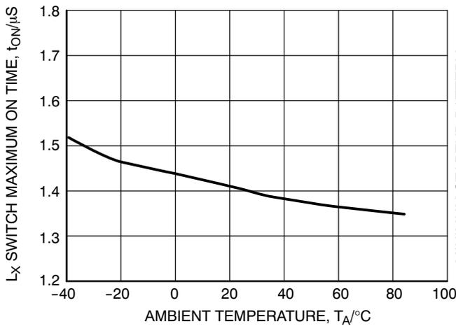
Figure 7. L<sub>X</sub> Switch Maximum ON Time vs. Temperature
