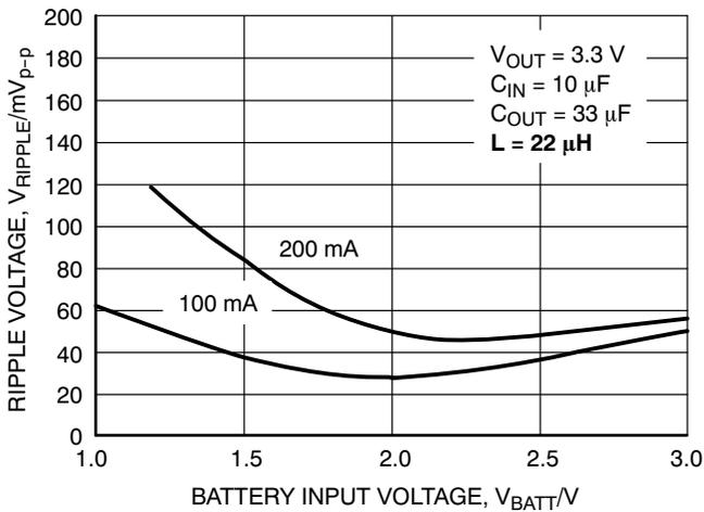
Figure 17. Output Ripple Voltage vs. Battery Input Voltage
