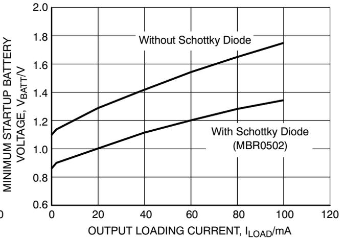
Figure 8. Minimum Startup Battery Voltage vs. Loading Current
