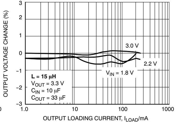
Figure 16. Output Voltage Change vs. Load Current
