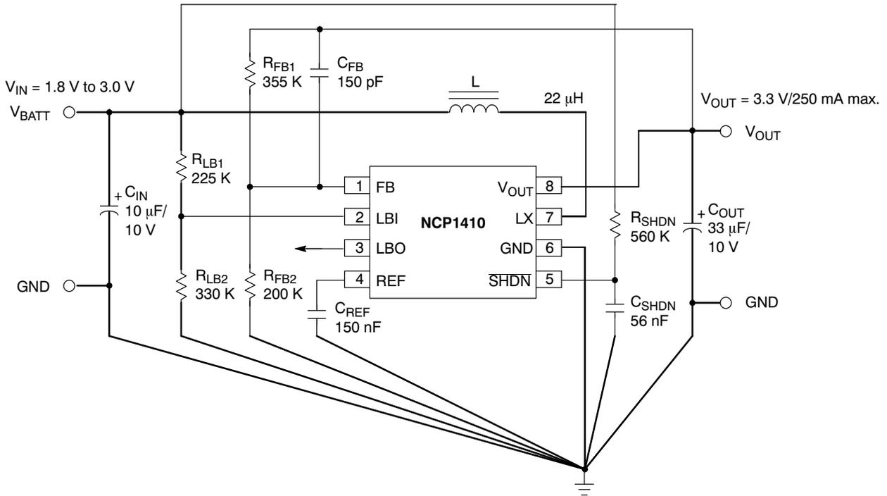
Figure 28. Typical Application Schematic for 2 Alkaline Cells Supply
