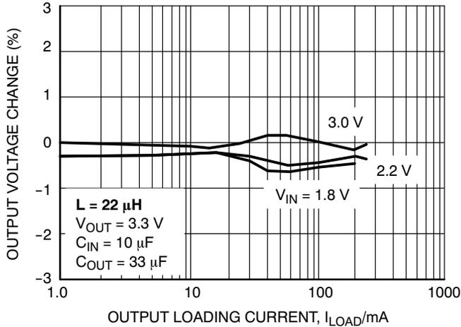
Figure 15. Output Voltage Change vs. Load Current
