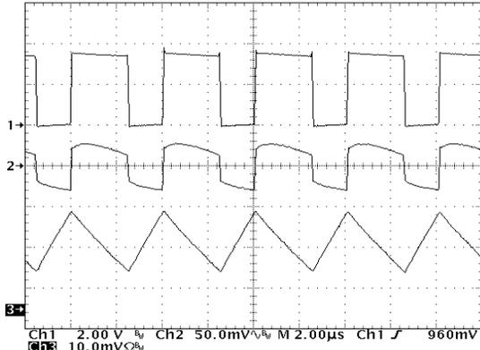
( $V_{IN} = 2.2\text{ V}$ ,  $V_{OUT} = 3.3\text{ V}$ ,  $I_{LOAD} = 10\text{ mA}$ ;  $L = 22\text{ }\mu\text{H}$ ,  $C_{OUT} = 33\text{ }\mu\text{F}$ )
