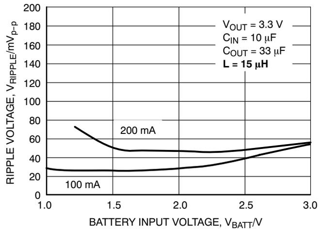
Figure 18. Output Ripple Voltage vs. Battery Input Voltage
