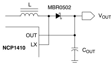
Figure 27. Schottky Device Between LX and OUT Pins
