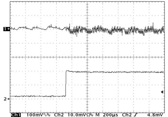
( $V_{OUT} = 3.3\text{ V}$ ,  $I_{LOAD} = 10\text{ mA}$  to  $100\text{ mA}$ ;  $L = 22\text{ }\mu\text{H}$ ,  $C_{OUT} = 33\text{ }\mu\text{F}$ )
