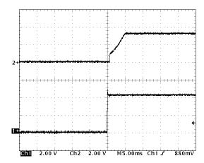
$\begin{aligned} (V_{IN} = 4.3 \text{ V, } V_{OUT} = 3.3 \text{ V, } C_{SS} = 100 \text{ pF, No load}) \\ \text{Upper Trace: Output Voltage, } 2.0 \text{ V/Div.} \\ \text{Lower Trace: EN Pin Waveform, } 2.0 \text{ V/Div.} \\ \text{Time Scale: } 5.0 \text{ ms/Div.} \end{aligned}$
