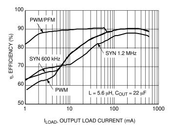
Figure 19. Efficiency vs. Output Load Current (V<sub>IN</sub> = 4.0 V, V<sub>OUT</sub> = 3.0 V)
