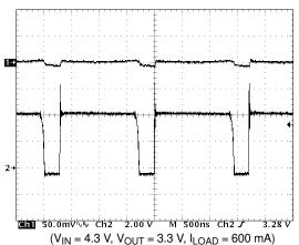
Upper Trace: Output Voltage Ripple, 50 mVac/Div. Lower Trace: LX Pin Switching Waveform, 2.0 V/Div.
