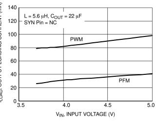
Figure 12. PWM/PFM Switchover Current Thresholds vs. Input Voltage (V<sub>OUT</sub> = 2.7 V)
