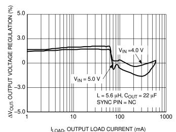
Figure 25. Output Voltage Regulation vs. Output Load Current (V<sub>OUT</sub> = 3.0 V)
