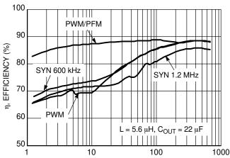
I<sub>LOAD</sub>, OUTPUT LOAD CURRENT (mA)
