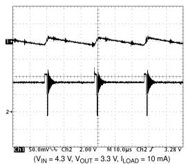
Upper Trace: Output Voltage Ripple, 50 mVac/Div. Lower Trace: LX Pin Switching Waveform, 2.0 V/Div.
