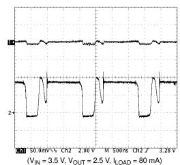
Upper Trace: Output Voltage Ripple, 50 mVac/Div. Lower Trace: LX Pin Switching Waveform, 2.0 V/Div.
