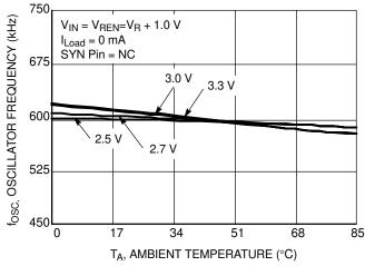
Figure 9. Oscillator Frequency vs. Ambient Temperature
