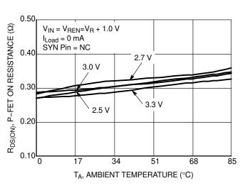
Figure 10. P-FET ON Resistance vs. Ambient Temperature
