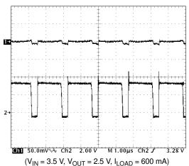
Upper Trace: Output Voltage Ripple, 50 mVac/Div.
