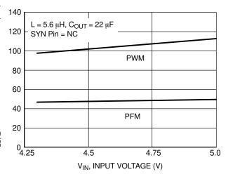
Figure 14. PWM/PFM Switchover Current Thresholds vs. Input Voltage (V<sub>OUT</sub> = 3.3 V)
