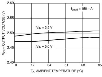
Figure 3. Output Voltage vs. Ambient Temperature (V<sub>OUT</sub> = 2.5 V)
