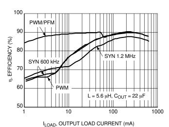
Figure 17. Efficiency vs. Output Load Current (V<sub>IN</sub> = 3.7 V, V<sub>OUT</sub> = 2.7 V)
