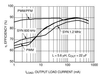
Figure 15. Efficiency vs. Output Load Current (V<sub>IN</sub> = 3.5 V, V<sub>OUT</sub> = 2.5 V)
