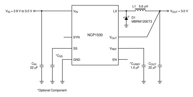
Figure 1. Typical Step-Down Converter Application
