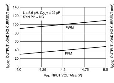
Figure 13. PWM/PFM Switchover Current Thresholds vs. Input Voltage (V<sub>OUT</sub> = 3.0 V)
