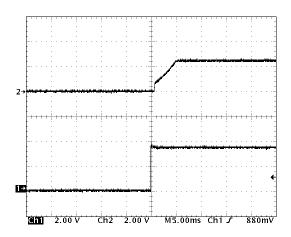
(V<sub>IN</sub> = 3.5 V, V<sub>OUT</sub> = 2.5 V, C<sub>SS</sub> = 100 pF, No load) Upper Trace: Output Voltage, 2.0 V/Div. Lower Trace: EN Pin Waveform, 2.0 V/Div. Time Scale: 5.0 ms/Div.
