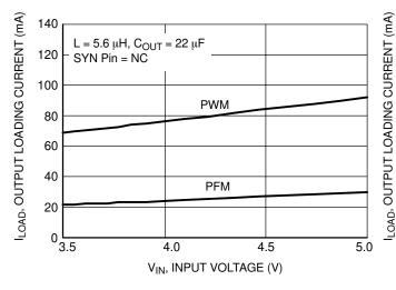
Figure 11. PWM/PFM Switchover Current Thresholds vs. Input Voltage (V<sub>OUT</sub> = 2.5 V)
