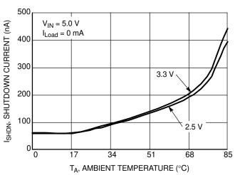
Figure 7. Supply Current vs. Ambient Temperature
