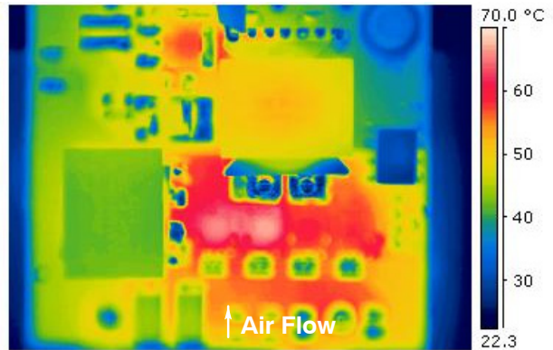
Figure 36. Thermal Image of the Top of the Board at High Line and Full Load Condition
