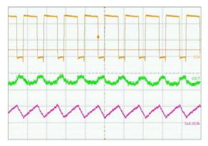
$\begin{array}{l} (V_{IN}=5 \ V, \ I_{LOAD}=700 \ mA, \ L=3.3 \ \mu H, \ C_{OUT}=2 \ x \ 22 \ \mu F) \\ Upper \ Trace: \ L_X \ Pin \ Switching \ Waveform, \ 2 \ V/div \\ Middle \ Trace: \ Output \ Ripple \ Voltage, \ 20 \ mV/div \\ Lower \ Trace: \ Inductor \ Current, \ 1 \ A/div \\ Time \ Scale: \ 1.0 \ \mu s/div \end{array}$
