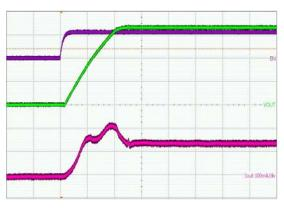
$(V_{IN} = 5 \text{ V}, I_{LOAD} = 100 \text{ mA}, L = 3.3 \ \mu\text{H}, C_{OUT} = 2 \ x \ 22 \ \mu\text{F}) \\ Upper Trace: EN Pin Voltage, 2 V/div \\ Middle Trace: Output Voltage, 1 V/div \\ Lower Trace: Inductor Current, 100 mA/div \\ Time Scale: 500 \ \mu\text{s/div} \\ Figure 19. Soft-Start Waveforms for V_{OUT} = 3.3 \ V \\$
