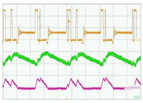
$\begin{array}{l} (V_{IN}=5 \ V, \ I_{LOAD}=100 \ mA, \ L=3.3 \ \mu\text{H}, \ C_{OUT}=2 \ x \ 22 \ \mu\text{F}) \\ \text{Upper Trace: } L_X \ \text{Pin Switching Waveform, } 2 \ V/div \\ \text{Middle Trace: Output Ripple Voltage, } 20 \ mV/div \\ \text{Lower Trace: Inductor Current, } 200 \ mA/div \\ \text{Time Scale: } 1.0 \ \mu\text{s/div} \end{array}$
