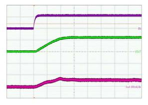
$(V_{IN} = 5 \text{ V}, \text{ I}_{LOAD} = 100 \text{ mA}, \text{ L} = 3.3 \ \mu\text{H}, \text{ C}_{OUT} = 2 \ x \ 22 \ \mu\text{F} ) \\ \text{Upper Trace: EN Pin Voltage, 2 V/div} \\ \text{Middle Trace: Output Voltage, 1 V/div} \\ \text{Lower Trace: Inductor Current, 100 mA/div} \\ \text{Time Scale: 500 } \mu\text{s/div} \\ \text{Figure 20. Soft-Start Waveforms for V}_{OUT} = 1.2 \ \text{V}$
