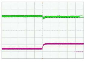
$(V_{IN} = 5 \ V, \ I_{LOAD} = 100 \ mA, \ L = 3.3 \ H, \ C_{OUT} = 2 \ x \ 22 \ \mu F) \\ Upper Trace: Output Dynamic Voltage, 100 mV/div \\ Lower Trace: Output Current, 500 mA/div \\ Time Scale: 200 \ \mu s/div$
