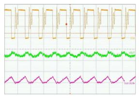
$\begin{array}{l} (V_{IN}=5 \; V, \; I_{LOAD}=100 \; mA, \; L=3.3 \; \mu H, \; C_{OUT}=2 \; x \; 22 \; \mu F) \\ \text{Upper Trace: } L_X \; \text{Pin Switching Waveform, } 2 \; V/div \\ \text{Middle Trace: Output Ripple Voltage, } 20 \; mV/div \\ \text{Lower Trace: Inductor Current, } 1 \; A/div \\ \text{Time Scale: } 1.0 \; \mu \text{s/div} \end{array}$
