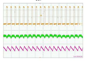
$(V_{IN} = 5 \text{ V, } I_{LOAD} = 400 \text{ mA, } L = 3.3 \mu\text{H}, C_{OUT} = 2 \text{ x } 22 \mu\text{F} ) \\ Upper Trace: L_X Pin Switching Waveform, 2 V/div \\ Middle Trace: Output Ripple Voltage, 20 mV/div \\ Lower Trace: Inductor Current, 1 A/div \\ Time Scale: 1.0 \mu\text{s/div}$
