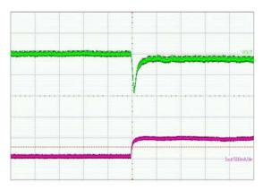
$\begin{array}{l} (V_{IN}=5~V, I_{LOAD}=100~mA, L=3.3~\mu H, C_{OUT}=2~x~22~\mu F)\\ Upper Trace: Output Dynamic Voltage, 100~mV/div\\ Lower Trace: Output Current, 500~mA/div\\ Time~Scale: 200~\mu s/div \end{array}$
