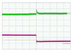
$\begin{array}{l} (V_{IN}=5 \ V, \ I_{LOAD}=100 \ mA, \ L=3.3 \ H, \ C_{OUT}=2 \ x \ 22 \ \mu F) \\ Upper \ Trace: \ Output \ Dynamic \ Voltage, \ 100 \ mV/div \\ Lower \ Trace: \ Output \ Current, \ 500 \ mA/div \\ Time \ Scale: \ 200 \ \mu s/div \end{array}$
