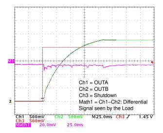
Figure 30. Zero Pop Noise Turn On Sequence with Differential Input to Ground; C<sub>in</sub> = 100 nF, R<sub>in</sub> = 24  $\Omega$ , R<sub>f</sub> = 100 k $\Omega$ , C<sub>byp</sub> = 1  $\mu$ F, R<sub>L</sub> = 8  $\Omega$
