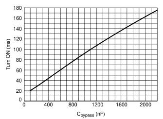
Figure 21.  $T_{ON}$  versus  $C_{bypass}$  @  $V_{bat}$  = 3.6 V,  $T_A$  = +25°C
