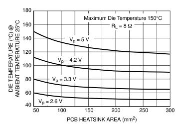
Figure 29. Maximum Die Temperature versus PCB Heatsink Area
