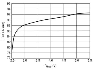
Figure 23.  $T_{ON}$  vs.  $V_{bat}$  @  $C_{bypass}$  = 1  $\mu F$ ,  $T_A$  = +25°C
