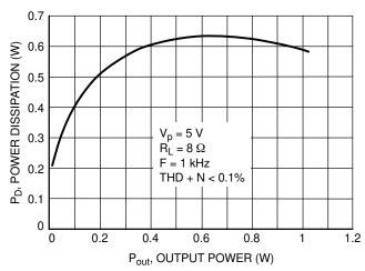
Figure 24. Power Dissipation versus Output Power
