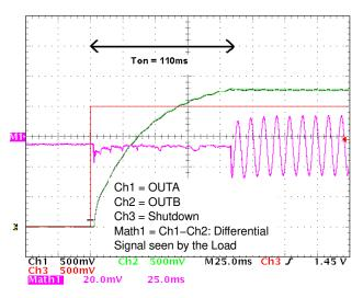
Figure 31. Zero Pop Noise Turn On Sequence with Differential Audio Source;  $C_{in}$  = 100 nF,  $R_{in}$  = 24  $\Omega$ ,  $R_f$  = 100 k $\Omega$ ,  $C_{byp}$  = 1  $\mu$ F,  $R_L$  = 8  $\Omega$
