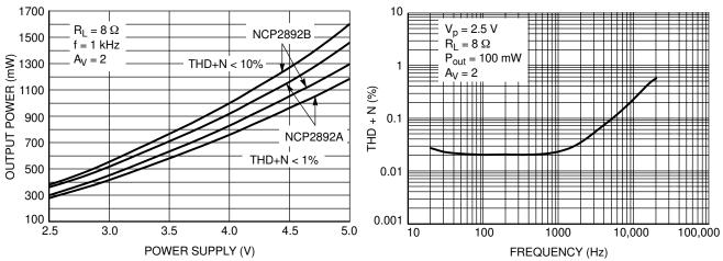
Figure 9. Output Power versus Power Supply
