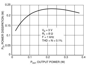
Figure 26. Power Dissipation versus Output Power
