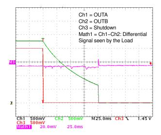
Figure 32. Zero Pop Noise Turn Off Sequence with Differential Input to Ground;  $C_{in}$  = 100 nF,  $R_{in}$  = 24  $\Omega$ ,  $R_f$  = 100 k $\Omega$ ,  $C_{byp}$  = 1  $\mu$ F,  $R_L$  = 8  $\Omega$
