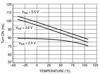
Figure 22.  $T_{ON}$  versus Temperature @  $V_{bat}$  = 3.6 V,  $C_{bypass}$  = 1  $\mu F$
