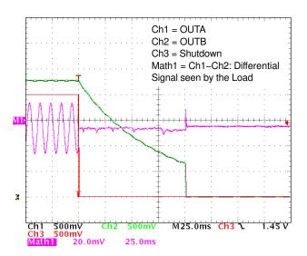
Figure 33. Zero Pop Noise Turn Off Sequence with Differential Audio Source;  $C_{in}$  = 100 nF,  $R_{in}$  = 24  $\Omega$ ,  $R_{f}$  = 100 k $\Omega$ ,  $C_{byp}$  = 1  $\mu$ F,  $R_{L}$  = 8  $\Omega$
