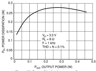
Figure 25. Power Dissipation versus Output Power
