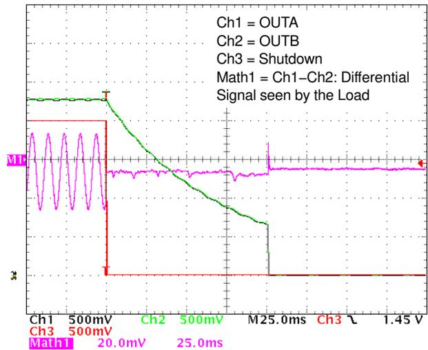
Figure 33. Zero Pop Noise Turn Off Sequence with Differential Audio Source;  $C_{in} = 100 \text{ nF}$ ,  $R_{in} = 24 \Omega$ ,  $R_f = 100 \text{ k}\Omega$ ,  $C_{byp} = 1 \mu\text{F}$ ,  $R_L = 8 \Omega$
