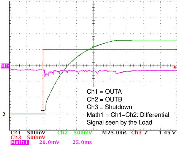
Figure 30. Zero Pop Noise Turn On Sequence with Differential Input to Ground;  $C_{in} = 100 \text{ nF}$ ,  $R_{in} = 24 \Omega$ ,  $R_f = 100 \text{ k}\Omega$ ,  $C_{byp} = 1 \mu\text{F}$ ,  $R_L = 8 \Omega$
