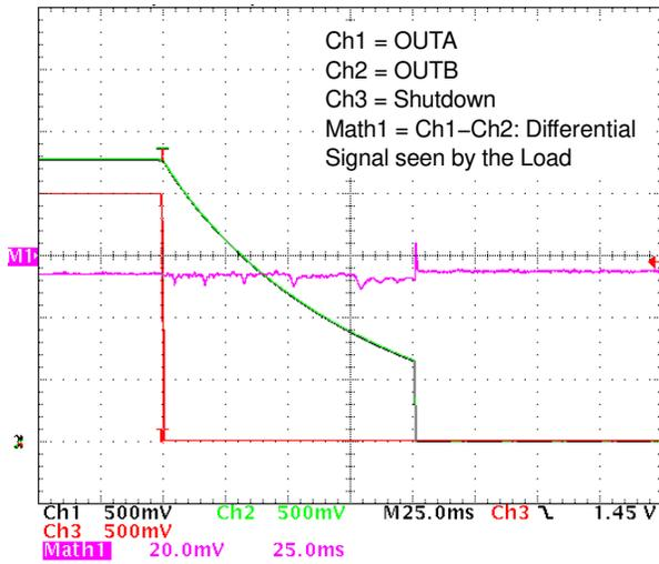
Figure 32. Zero Pop Noise Turn Off Sequence with Differential Input to Ground;  $C_{in} = 100 \text{ nF}$ ,  $R_{in} = 24 \Omega$ ,  $R_f = 100 \text{ k}\Omega$ ,  $C_{byp} = 1 \mu\text{F}$ ,  $R_L = 8 \Omega$
