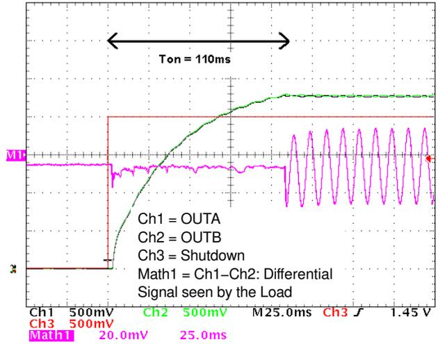
Figure 31. Zero Pop Noise Turn On Sequence with Differential Audio Source;  $C_{in} = 100 \text{ nF}$ ,  $R_{in} = 24 \Omega$ ,  $R_f = 100 \text{ k}\Omega$ ,  $C_{byp} = 1 \mu\text{F}$ ,  $R_L = 8 \Omega$
