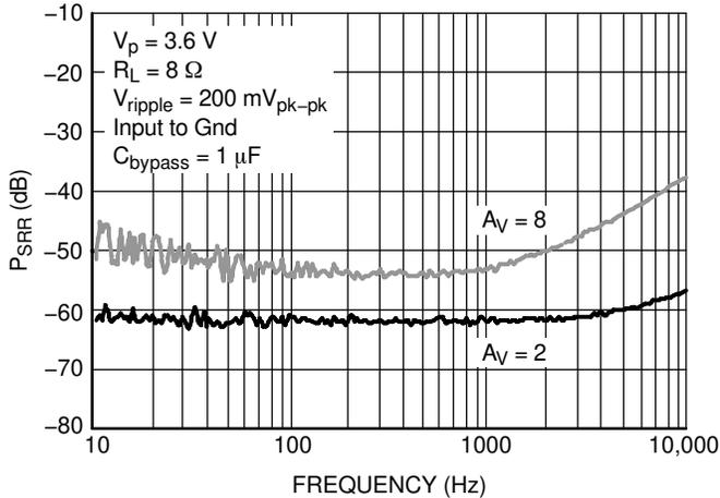
**Figure 15. PSRR @  $V_p = 3.6\text{ V}$
