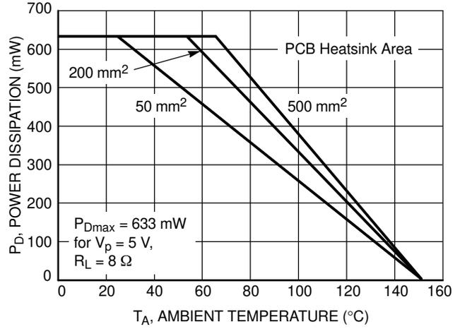
Figure 28. Power Derating - 9-Pin Flip-Chip CSP
