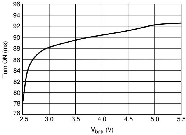
Figure 23.  $T_{ON}$  vs.  $V_{bat}$  @  $C_{bypass} = 1 \mu\text{F}$ ,  $T_A = +25^\circ\text{C}$
