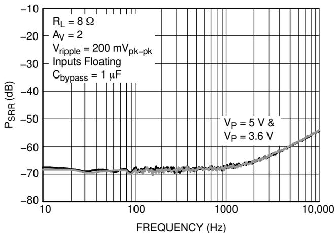
**Figure 19. PSRR @  $V_p = 3.6\text{ V}$
