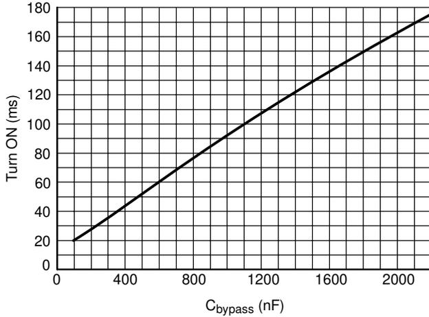
Figure 21.  $T_{ON}$  versus  $C_{bypass}$  @  $V_{bat} = 3.6$  V,  $T_A = +25^\circ\text{C}$
