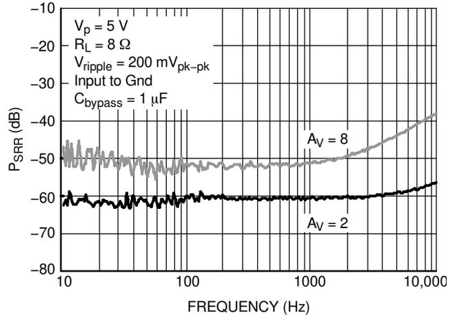
**Figure 16. PSRR @  $V_p = 5\text{ V}$
