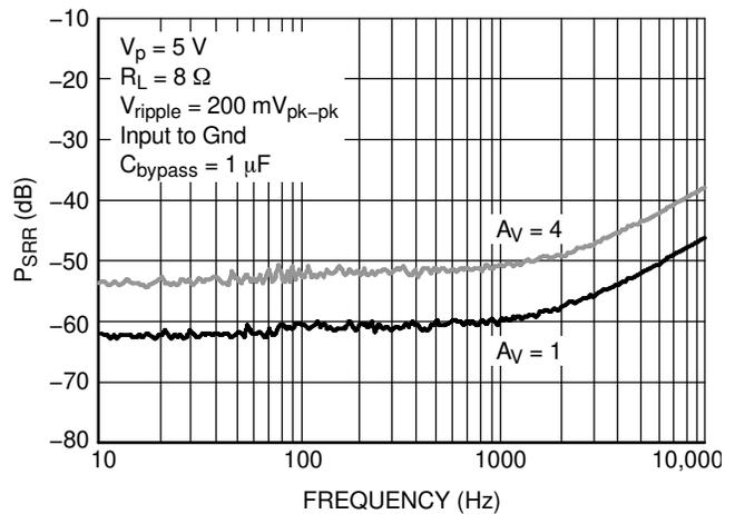
**Figure 18. PSRR @  $V_p = 5\text{ V}$
