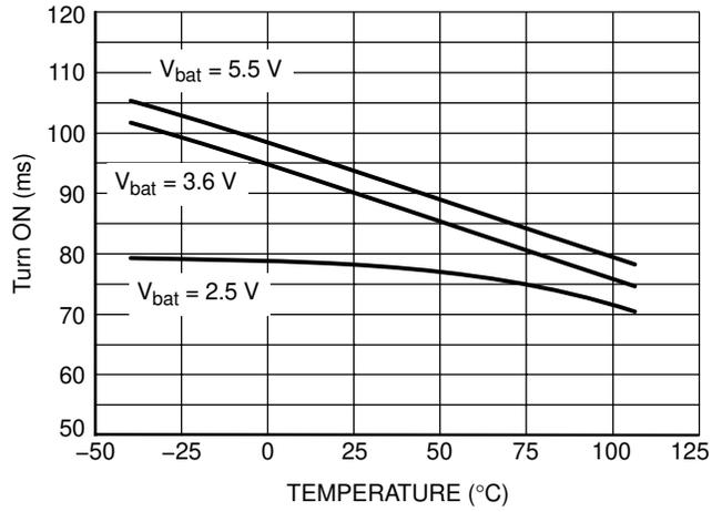
Figure 22.  $T_{ON}$  versus Temperature @  $V_{bat} = 3.6$  V,  $C_{bypass} = 1 \mu\text{F}$
