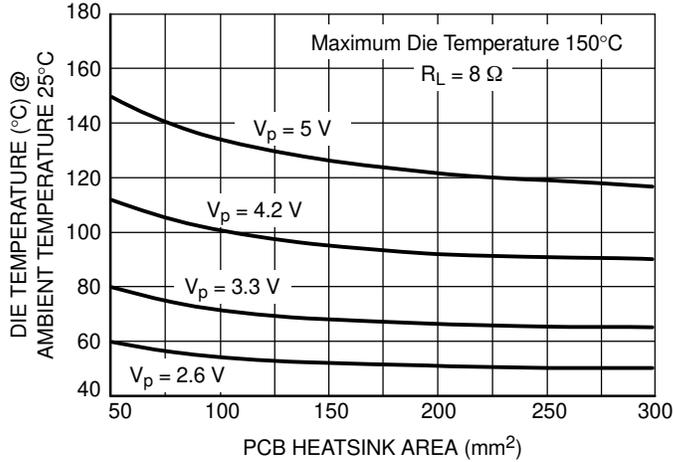
Figure 29. Maximum Die Temperature versus PCB Heatsink Area
