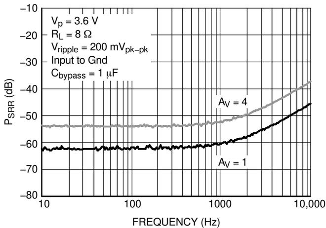
**Figure 17. PSRR @  $V_p = 3.6\text{ V}$
