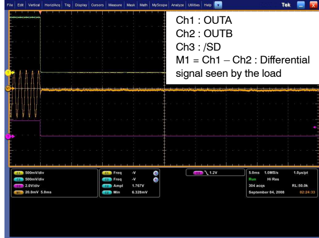
Figure 36. Zero pop noise turn off sequence with single-ended input audio source ( C_i = 47 \text{ nF} , R_i = 24 \text{ k}\Omega , R_f = 24 \text{ k}\Omega , C_{byp} = 1 \text{ }\mu\text{F} , R_l = 8 \text{ }\Omega , T_{on} = V_p )
