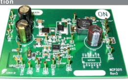
PowerGood pin to indicate that the system is in regulation. The dual function SYNC pin synchronizes the device to a higher frequency (Slave Mode) or outputs a 180° out-of-phase clock signal to drive another NCP3011 (Master Mode). Protection features include lossless current limit and short circuit protection, output overvoltage and undervoltage protection, and input undervoltage lockout.
