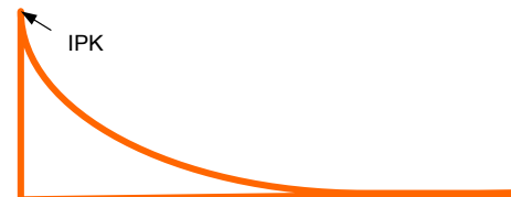
Figure 26. Input Charge Inrush Current
