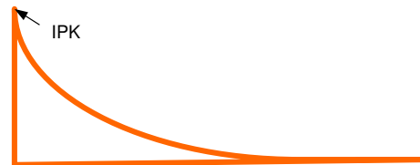
Figure 47. Input Charge Inrush Current
