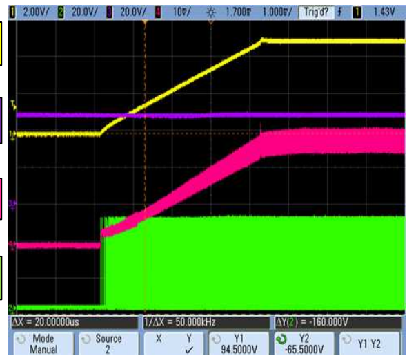
Figure 26. Start-Up Transition at 6A Load (EN = High)
