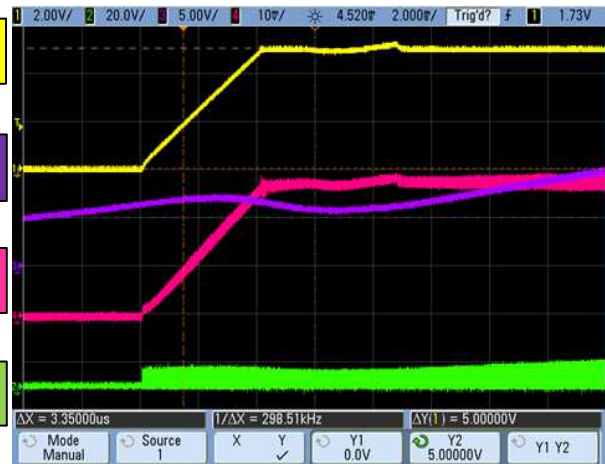
Figure 22. Start-Up Transition at 6A Load
