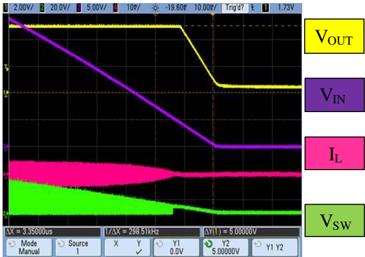
Figure 23. Shut-Down Transition at No Load
