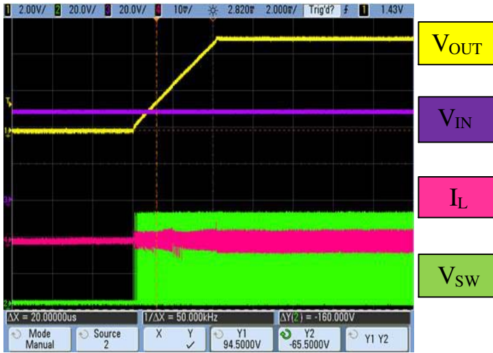
Figure 25. Start-Up Transition at No Load (EN = High)
