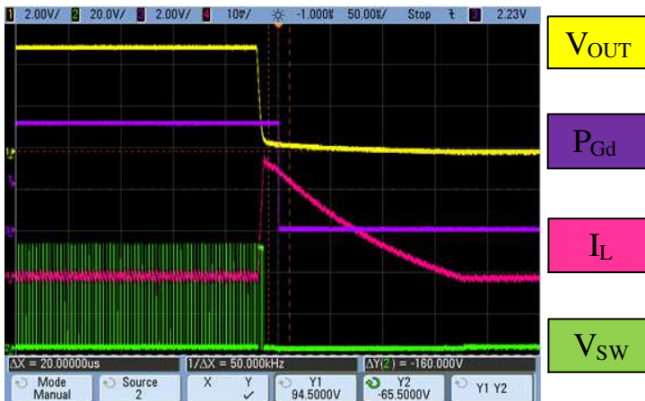
Figure 29. Short Circuit Test at No Load
