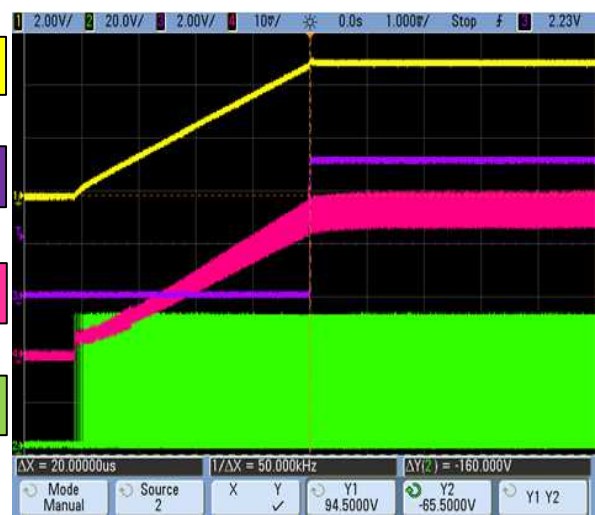
Figure 32. Recovery transition from Output Short at 6A Load
