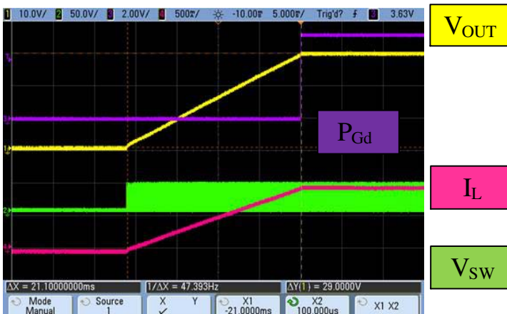
Figure 35. NCP4060 recovering from OTP
