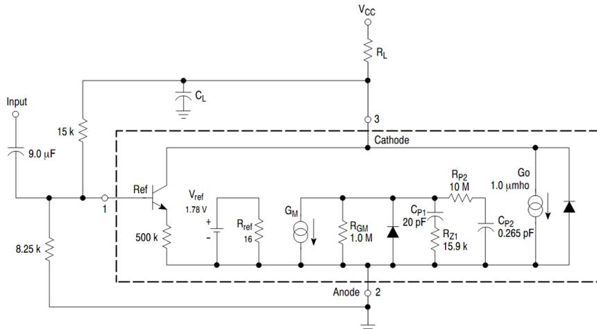
Figure 33. Simplified NCP431/NCP432 Device Model
