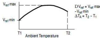
The average temperature coefficient of the reference input voltage, Vref is defined as:
