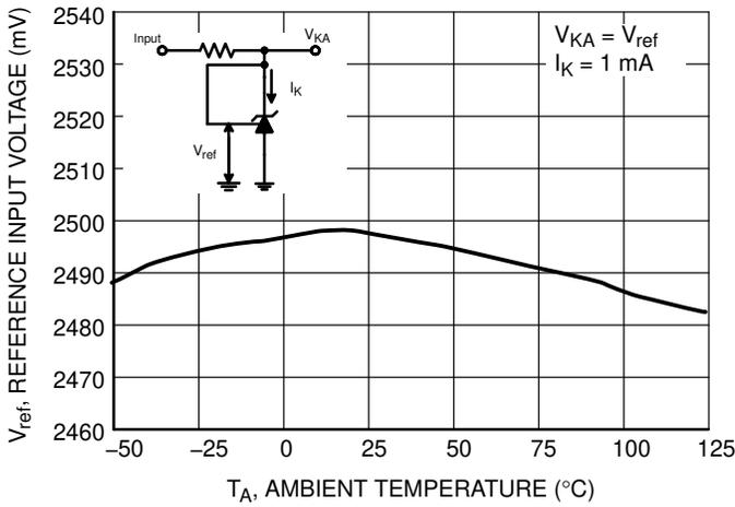
**Figure 9. Reference Input Voltage versus Ambient temperature**
