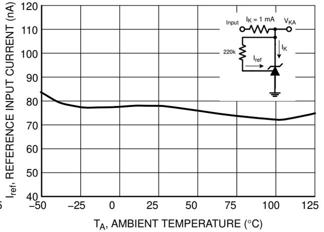
**Figure 10. Reference Input Current versus Ambient temperature**
