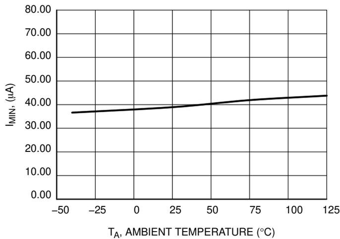
Figure 8. Minimum Cathode Current Regulation versus Ambient Temperature
