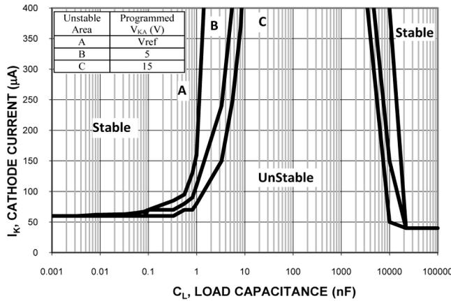
Figure 19. Stability Boundary Conditions for Small Cathode Current
