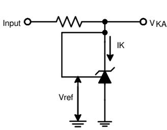
Figure 3. Test Circuit for  $V_{KA} = V_{ref}$
