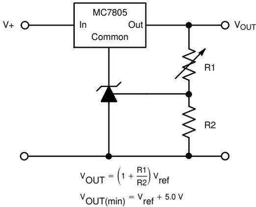
Figure 24. Output Control for a Tree-Terminal Fixed Regulator
