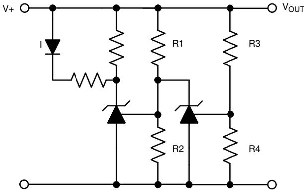
L.E.D. indicator is 'on' when  $V_+$  is between the upper and lower limits.
