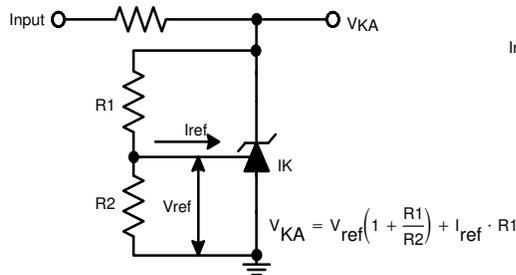
Figure 4. Test Circuit for  $V_{KA} > V_{ref}$
