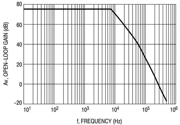
Figure 35. Example 2 Circuit Open Loop Gain Plot
