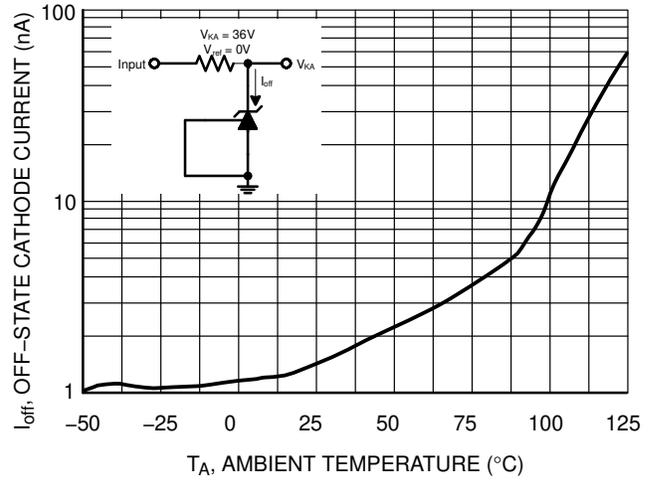
**Figure 12. Off-State Cathode Current versus Ambient Temperature**
