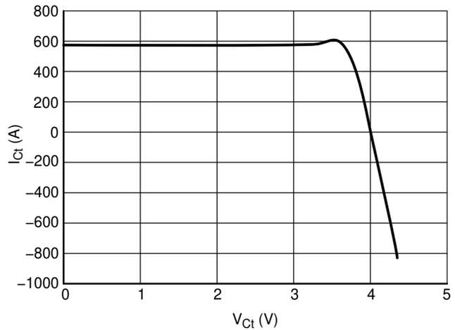
Figure 33. Internal Current Source on Ct Pin vs. V<sub>Ct</sub>
