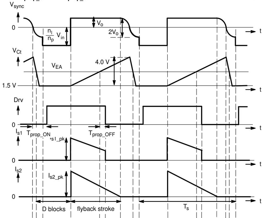
Figure 9.  $T_{prop\_ON}$  and  $T_{prop\_OFF}$  Timing Position in the Timing Application Diagram (in Normal Mode Operation)
