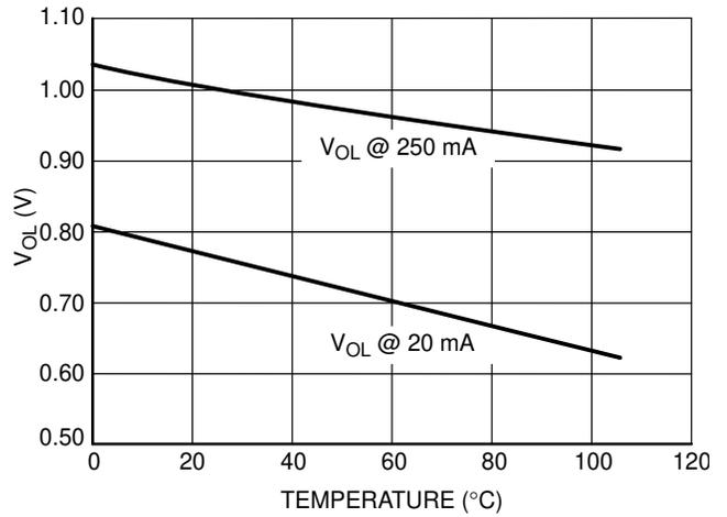
**Figure 11. Driver 1 Output Voltage Low State @ V<sub>CC</sub> = 15 V vs. Temperature**
