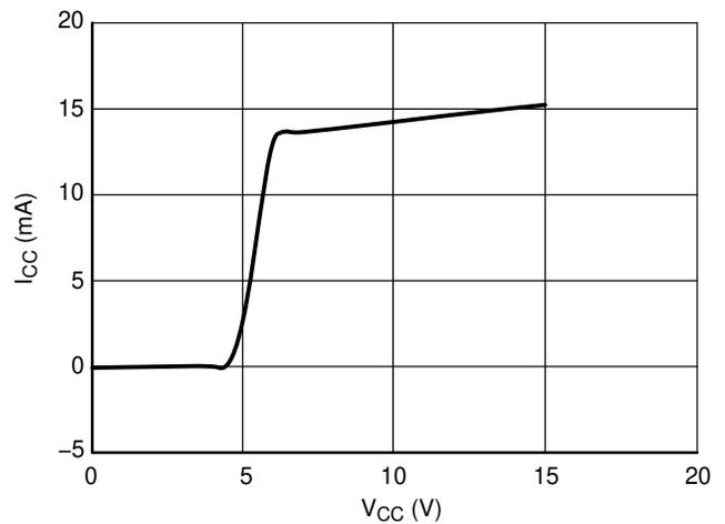
**Figure 38. Power Supply Current in Working Mode vs. Power Supply Voltage – V<sub>CC</sub>**
