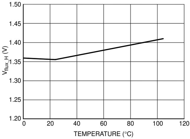
**Figure 22. High Level Flux Pin Clamp Voltage vs. Temperature**
