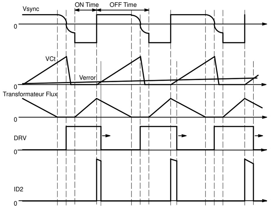
**Figure 43. Increasing Smoothly the Duty Cycle Does Not Yield a Smooth Peak Current Ramp up**
