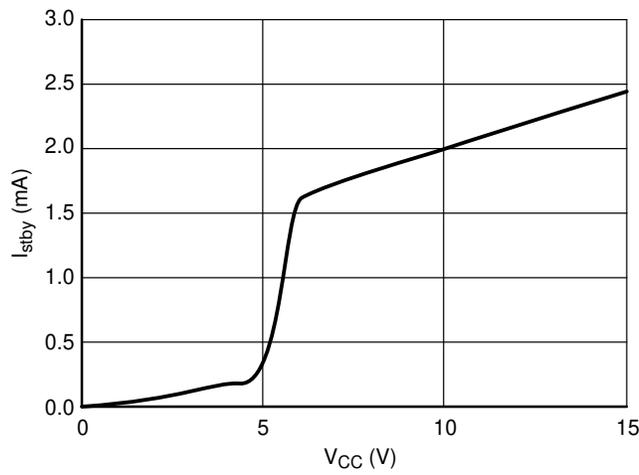
**Figure 36. Power Supply Current in Standby Mode vs. Power Supply Voltage – V<sub>CC</sub>**
