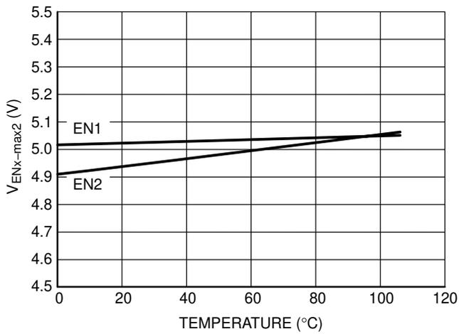
**Figure 18. Voltage on ENx Pin with an External Current Sink @ 500  $\mu$ A vs. Temperature**
