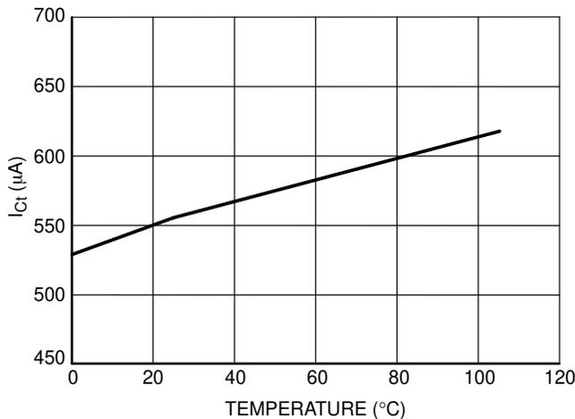
Figure 32. Internal Current Source on Ct Pin vs. Temperature
