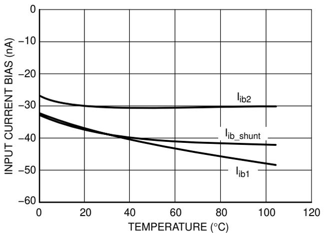
**Figure 27. Error Amplifier Input Bias Current vs. Temperature**
