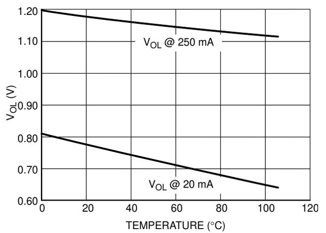
**Figure 13. Driver 2 Output Voltage Low State @ V<sub>CC</sub> = 15 V vs. Temperature**
