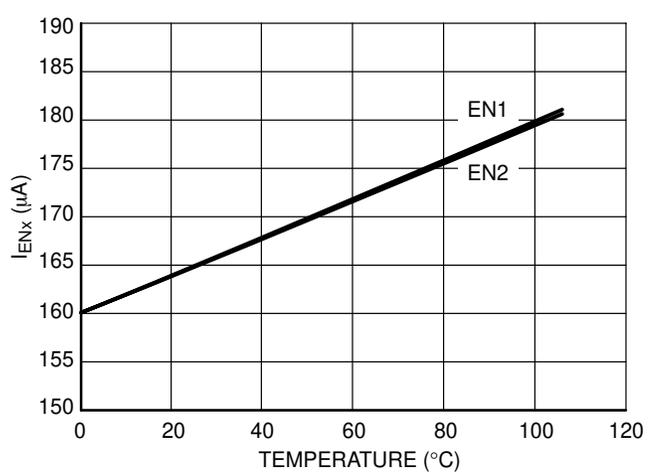
**Figure 15. Soft-Start Current Source on Enable Pin when V<sub>ENx</sub> = 2.5 V vs. Temperature**
