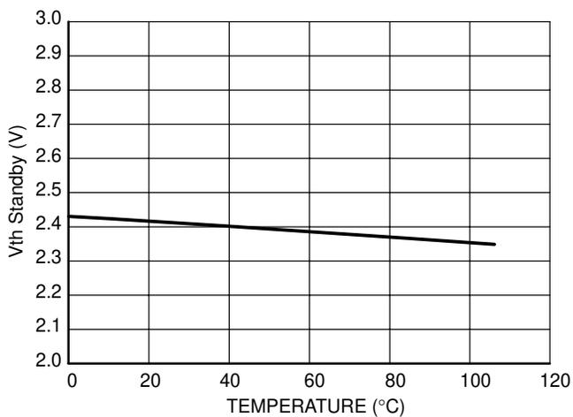
**Figure 14. Standby Pin Threshold Voltage vs. Temperature**
