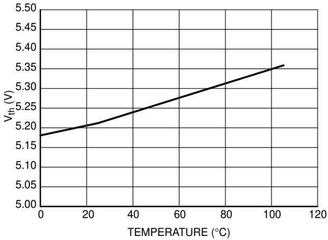
**Figure 34. Undervoltage Lockout, Startup Threshold vs. Temperature**
