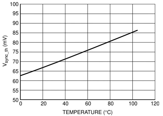
**Figure 25. Synchronization Input Voltage Threshold vs. Temperature**
