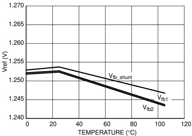
**Figure 26. Error Amplifier Internal Voltage Reference vs. Temperature**
