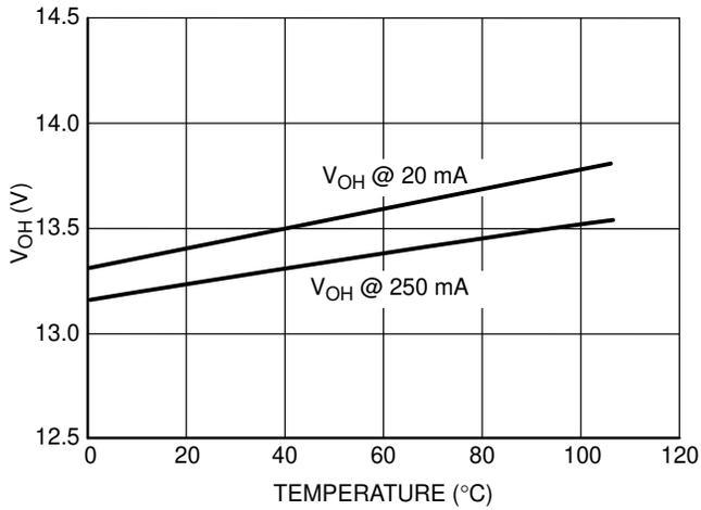
**Figure 10. Driver 1 Output Voltage High State @ V<sub>CC</sub> = 15 V vs. Temperature**
