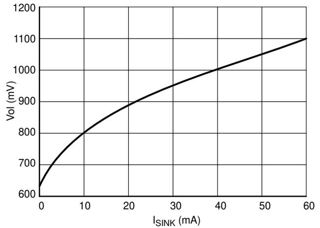
Figure 29. Error Amplifier Shunt Regulator Output Voltage Swing vs. Output Current (I<sub>SINK</sub>)
