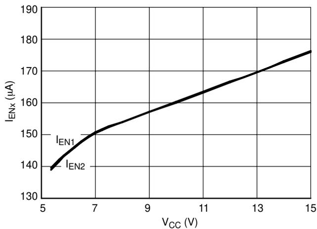
**Figure 20. Soft-Start Current Source on Enable Pin vs.  $V_{CC}$**
