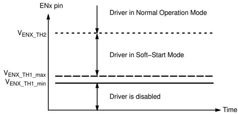
Figure 5. Enable Threshold Definition
