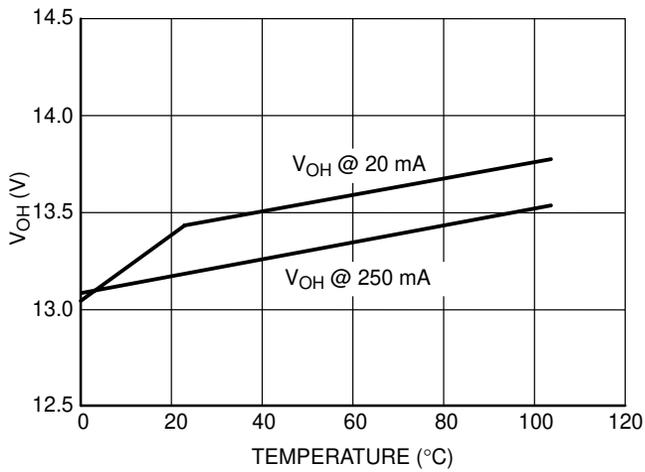
**Figure 12. Driver 2 Output Voltage High State @ V<sub>CC</sub> = 15 V vs. Temperature**
