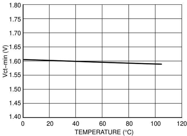
Figure 30. Minimum Voltage Clamp on Ct Pin vs. Temperature
