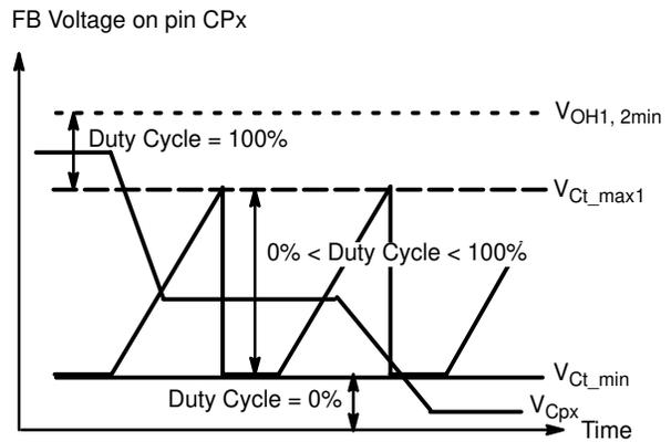
Figure 41. Duty Cycle Variation versus the Feedback Voltage
