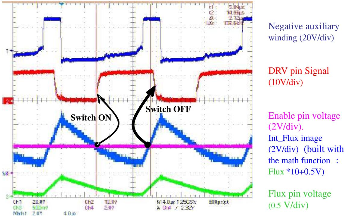
Figure 47. Soft-Start Duty Cycle Generation During the Startup Sequence
