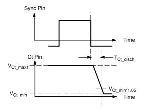
Figure 7. Discharging Time Definition (Ct Pin)
