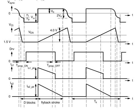
Figure 9. T<sub>prop\_ON</sub> and T<sub>prop\_OFF</sub> Timing Position in the Timing Application Diagram (in Normal Mode Operation)
