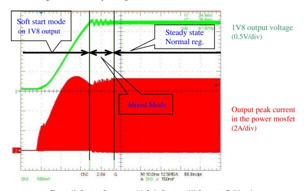
Figure 48. Startup Sequence with Soft-Start on 1V8 Output at Full Load
