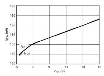
Figure 20. Soft–Start Current Source on Enable Pin vs. V<sub>CC</sub>
