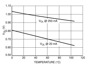
Figure 11. Driver 1 Output Voltage Low State
