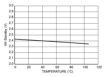
Figure 14. Standby Pin Threshold Voltage vs.
