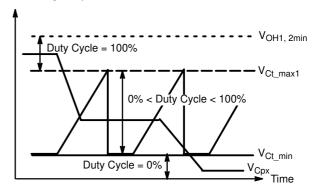
Figure 41. Duty Cycle Variation versus the Feedback Voltage
