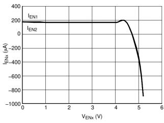
Figure 19. Soft-Start Current Source on Enable Pin vs. V<sub>EN</sub>
