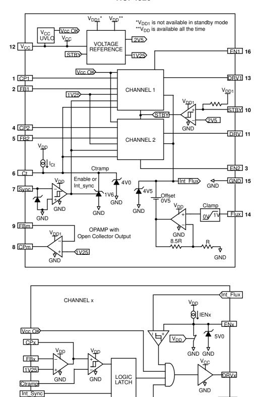
**Figure 3. Internal Circuit Architecture**
