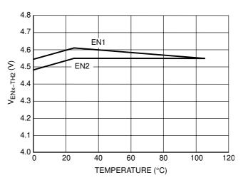
Figure 17. Max Voltage on ENx Pin Ending Soft-Start and Enable the Regulation Mode vs. Temperature
