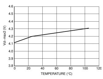
Figure 31. Maximum Voltage Clamp on Ct Pin @ 500 μA vs. Temperature
