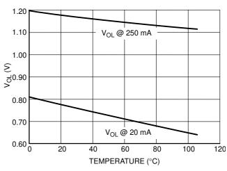
Figure 13. Driver 2 Output Voltage Low State
