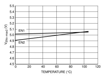
Figure 18. Voltage on ENx Pin with an External Current Sink @ 500 μA vs.
