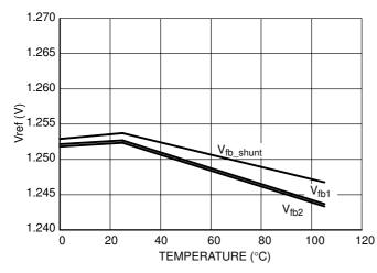
Figure 26. Error Amplifier Internal Voltage Reference vs. Temperature
