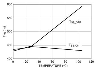
Figure 21. Turn ON and OFF Propagation Delay in Soft-Start Mode vs. Temperature
