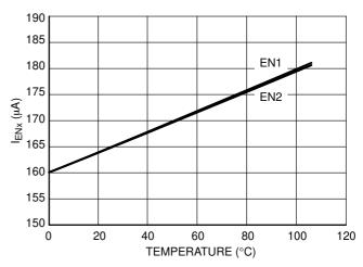
Figure 15. Soft–Start Current Source on Enable Pin when  $V_{ENx} = 2.5 \text{ V vs.}$  Temperature
