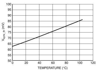
Figure 25. Synchronization Input Voltage Threshold vs. Temperature
