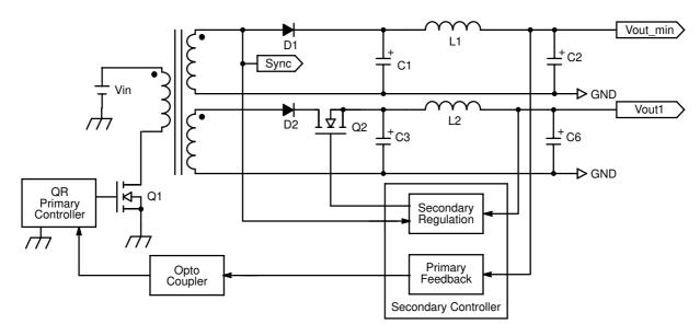
Figure 39. Regulation Principle Schematic
