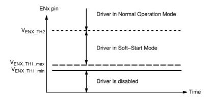
Figure 5. Enable Threshold Definition
