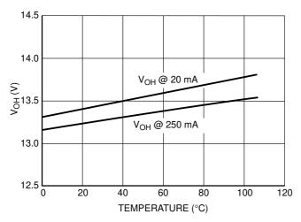
Figure 10. Driver 1 Output Voltage High State
