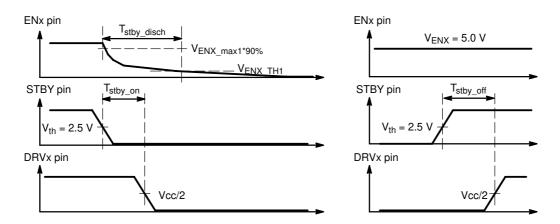
Figure 4. Standby Propagation Delay Definition
