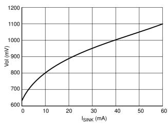
Figure 29. Error Amplifier Shunt Regulator Output Voltage Swing vs. Output Current (I<sub>sink</sub>)
