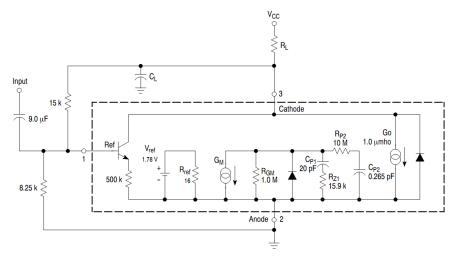
Figure 33. Simplified NCP431/NCP432 Device Model
