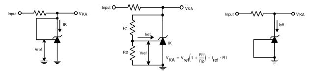
Figure 3. Test Circuit for  $V_{KA} = V_{ref}$
