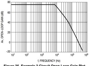
Figure 35. Example 2 Circuit Open Loop Gain Plot
