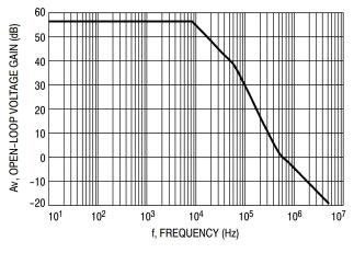
Figure 34. Example 1 Circuit Open Loop Gain Plot
