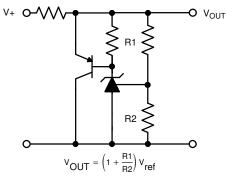
Figure 23. High Current Shunt Regulator
