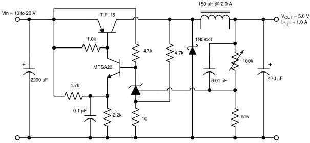
Figure 32. Step–Down Switching Converter
