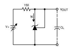
Figure 20. Test Circuit For Curve A of Stability Boundary Conditions
