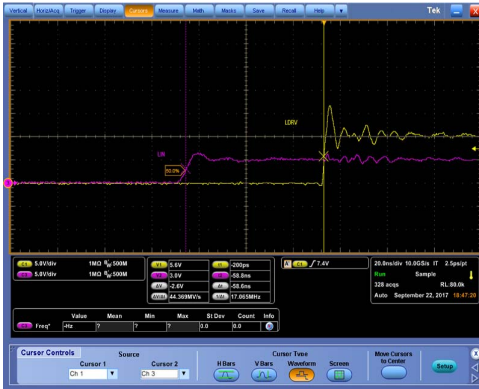
Figure 30. Low Side Turn-ON Propagation Delay (NCP51530A)
