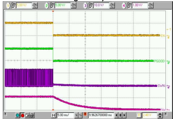
Top: EN2, CH2 Enable Signal, (5V/div) Middle 1: PGOOD2, CH2 Power Good Signal, (5V/div) Middle 2: SWN2, CH2 Switching Node Voltage, (10V/div) Bottom: Vo2, CH2 Output Voltage, (1V/div) Time: 5ms/div
