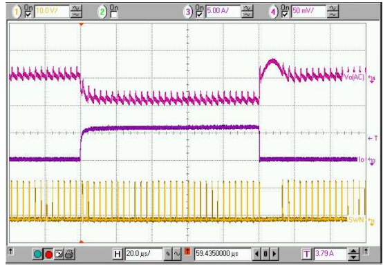
Top: Vo2, CH2 Output Voltage Ripple, (50mV/div) Middle: Io2, CH2 Output Current, (5A/div) Bottom: SWN2, CH2 Switching Node Voltage, (10V/div) Time: 20µs/div
