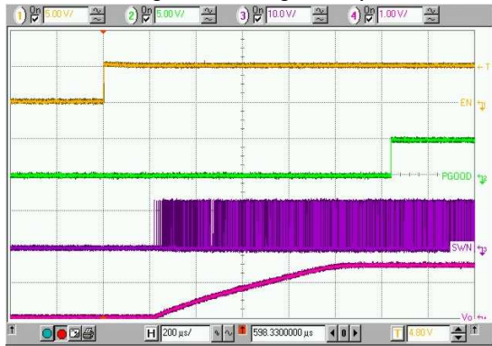
Top: EN1, CH1 Enable Signal, (5V/div) Middle 1: PGOOD1, CH1 Power Good Signal, (5V/div) Middle 2: SWN1, CH1 Switching Node Voltage, (10V/div) Bottom: Vo1, CH1 Output Voltage, (1V/div) Time: 200µs/div
