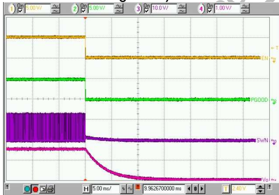
Top: EN1, CH1 Enable Signal, (5V/div) Middle 1: PGOOD1, CH1 Power Good Signal, (5V/div) Middle 2: SWN1, CH1 Switching Node Voltage, (10V/div) Bottom: Vo1, CH1 Output Voltage, (1V/div) Time: 5ms/div
