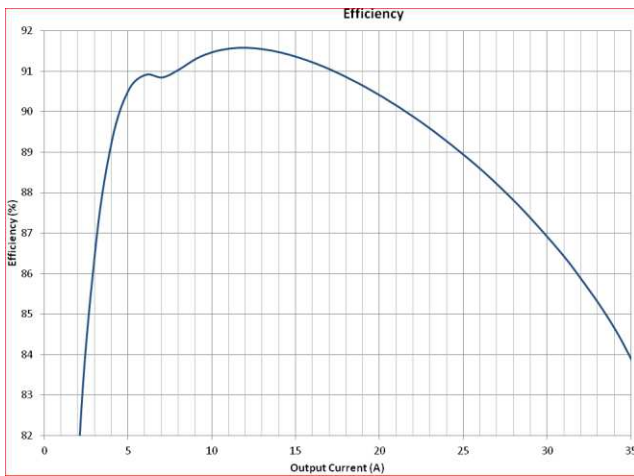
Figure 4. Efficiency – 12 V Input, 1.2 V Output, 500 kHz
