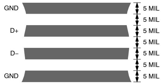
Figure 22. Typical Arrangement of Signal Tracks
