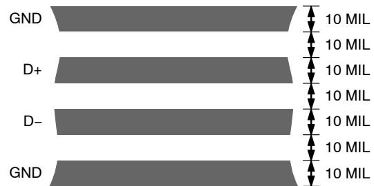
Figure 17. Arrangement of Signal Tracks
