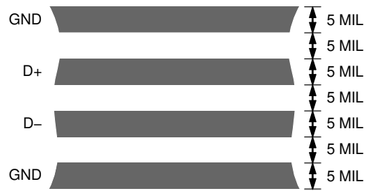
Figure 22. Typical Arrangement of Signal Tracks
