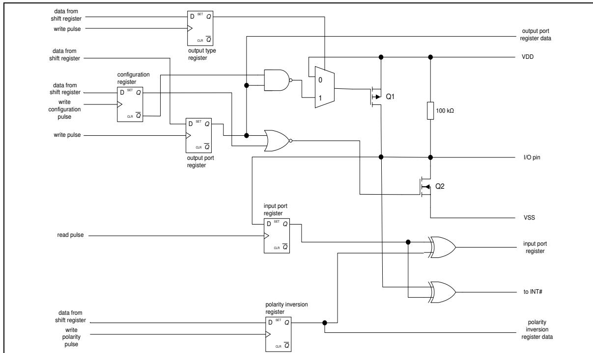
When an I/O is configured as an input (default), FETs Q1 and Q2 are off, creating a high-impedance input with a weak pull-up to VDD. The input voltage may be raised above VDD to a maximum of 5.5 V.
