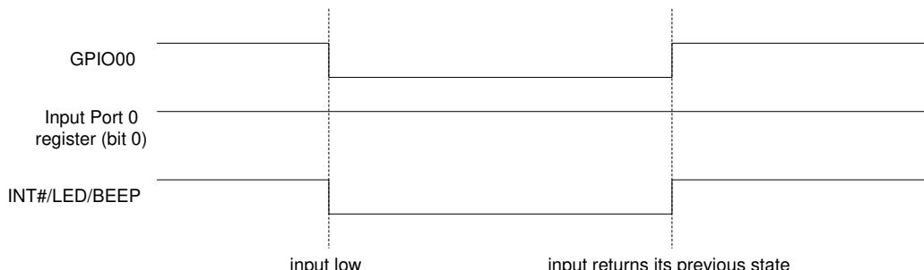
Example 3: GPIO00 input; polarity register set '0'; pulse output (Input Port register is read)
