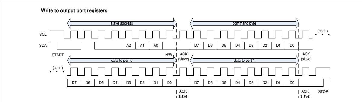
Data is transmitted to the NCT5655Y/W by sending the device address and setting the least significant bit to a logic 0. The command byte is sent after the address and determines which register will receive the data following the command byte.
