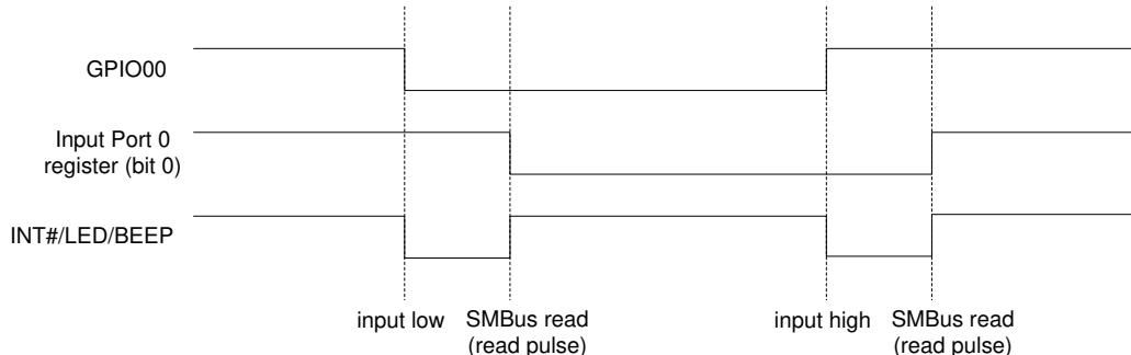
Example 2: GPIO00 input; polarity register set '0'; level output (input returns to its previous state)
