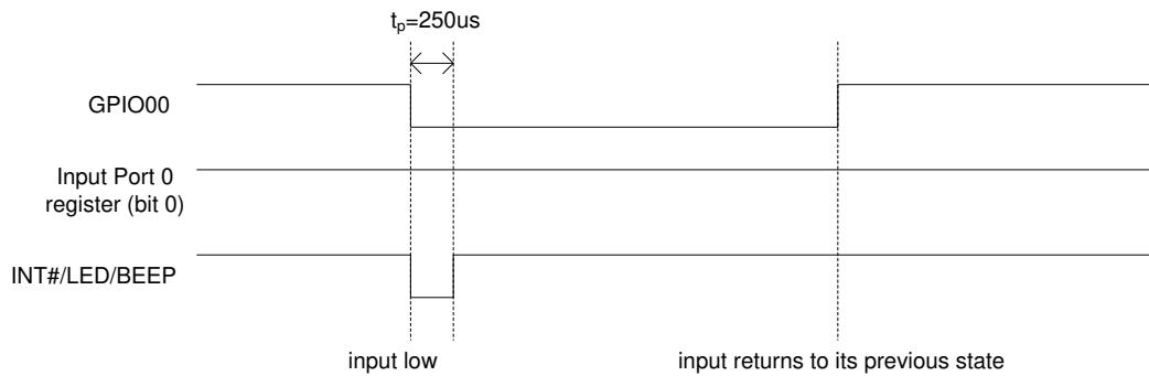
\*INT#/LED/BEEP output LED signal during low period when it is configured to LED output.
