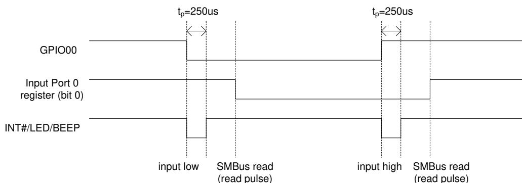
Example 4: GPIO00 input; polarity register set '0'; pulse output (input returns to its previous state)
