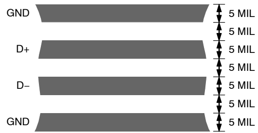
Figure 22. Typical Arrangement of Signal Tracks
