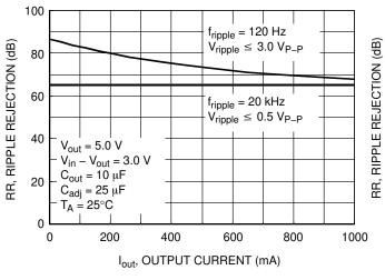
Figure 10. NCP1117XTA Ripple Rejection vs. Output Current
