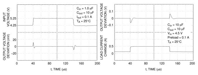
Figure 15. NCP1117XT285 Line Transient Response
