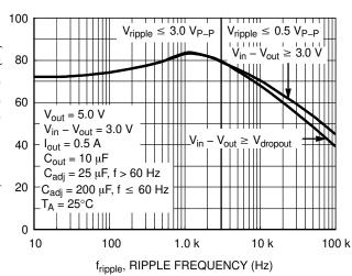
Figure 11. NCP1117XTA Ripple Rejection vs. Frequency
