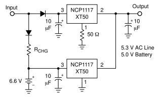
The 50  $\Omega$  resistor that is in series with the ground pin of the upper regulator level shifts its output 300 mV higher than the lower regulator. This keeps the lower regulator off until the input source is removed.
