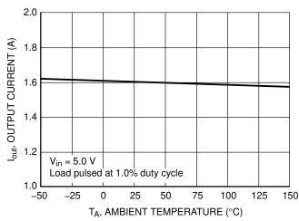
Figure 7. Output Short Circuit Current vs. Temperature
