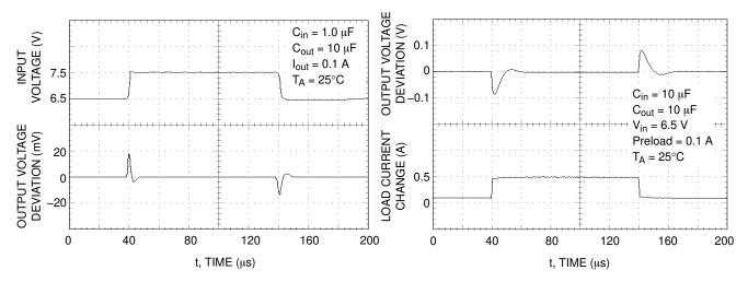
Figure 17. NCP1117XT50 Line Transient Response
