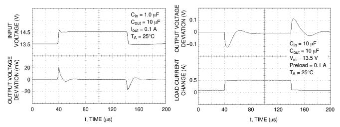
Figure 19. NCP1117XT12 Line Transient Response
