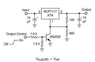
Figure 29. Regulator with Shutdown
