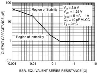
Figure 12. Output Capacitance vs. ESR
