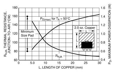
Figure 21. SOT–223 Thermal Resistance and Maximum Power Dissipation vs. P.C.B. Copper Length
