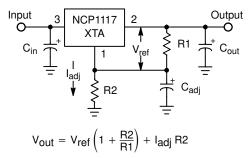
Figure 24. Adjustable Output Regulator
