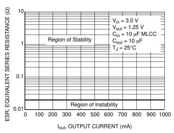
Figure 13. Typical ESR vs. Output Current
