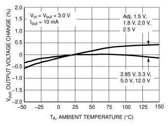
Figure 4. Output Voltage Change vs. Temperature
