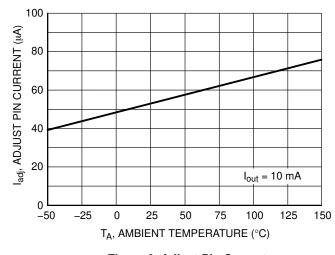
Figure 8. Adjust Pin Current vs. Temperature
