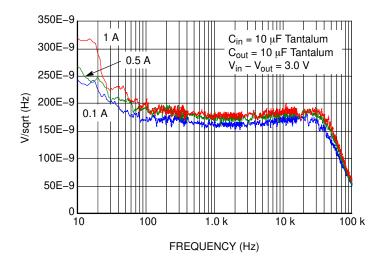
Figure 14. Output Spectral Noise Density vs. Frequency, V<sub>out</sub> = 1V5
