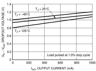
Figure 5. Dropout Voltage vs. Output Current
