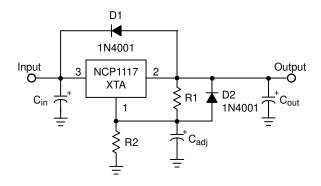
Figure 25. Protection Diode Placement
