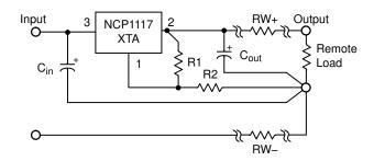
Figure 26. Load Sensing
