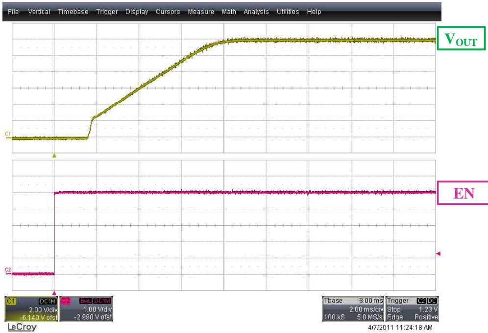
Figure 3. Typical Start-up with V_{IN} = 12\text{ V} , R_{OUT} = 6\ \Omega
